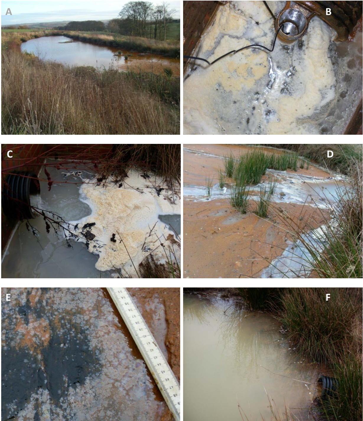
Figure 3 Contrary to RAPS 1, limited plant growth is observed on the RAPS 2 (Oct. 2007, A). Reddish and white staining are noted in the influent (B, C, D) and on the sediment surface. The increased precipitation of ochre sludge, especially around the inlet, causes a reduction of the free boards. At ~0.5 cm below surface (E) the colour of the sediment changes to black. Overflow pipe in RAPS 2 (F).
