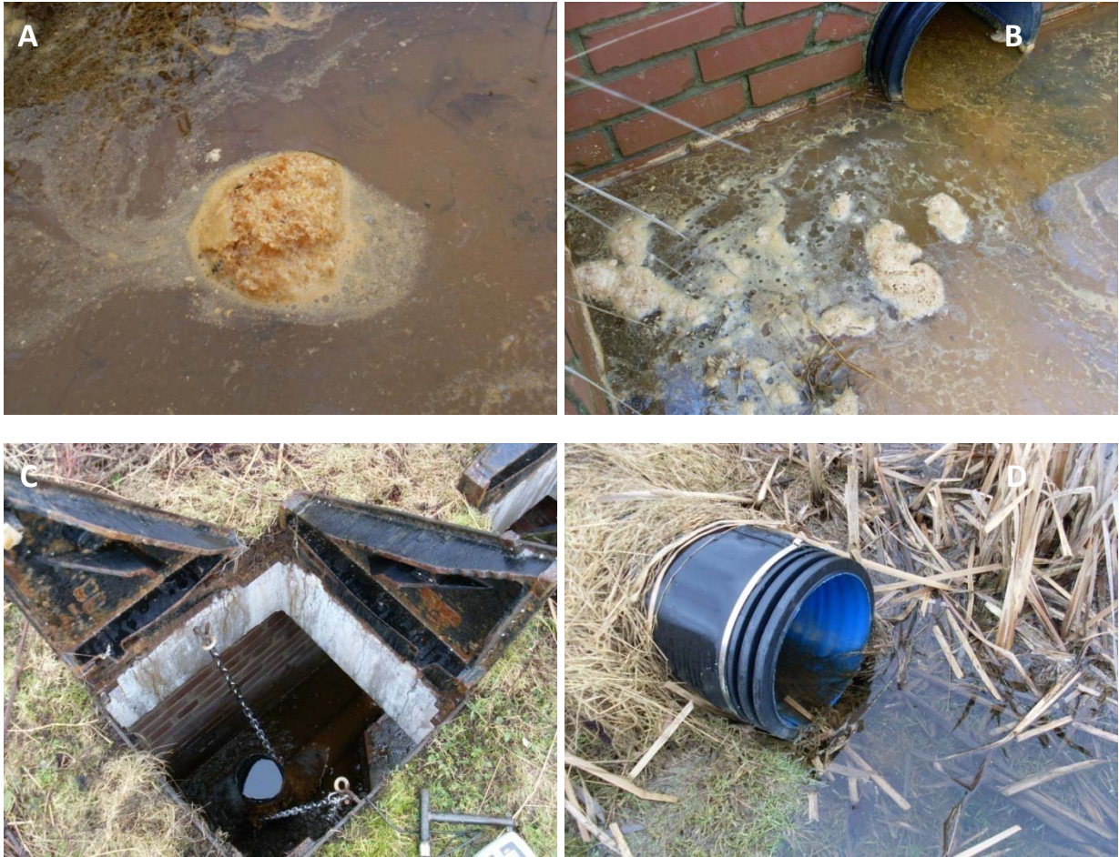
Figure 2 During January 2008 reddish (A) and greyish-white (B) froth was observable on the water surface of RAPS 1 near the inlet. Figure C shows the manhole chamber which collects RAPS 1 effluent water before discharge via a 58 m long subsurface drainage pipe into the polishing wetland. The effluent pipe is adjustable in order to control the height of the water cover overlying the reactive substrate (free board). In cases of high flow, a fraction of the water from the free board is discharged into the wetland via a subsurface overflow pipe (D), i.e. without having previously been in contact with the reactive substrate.
