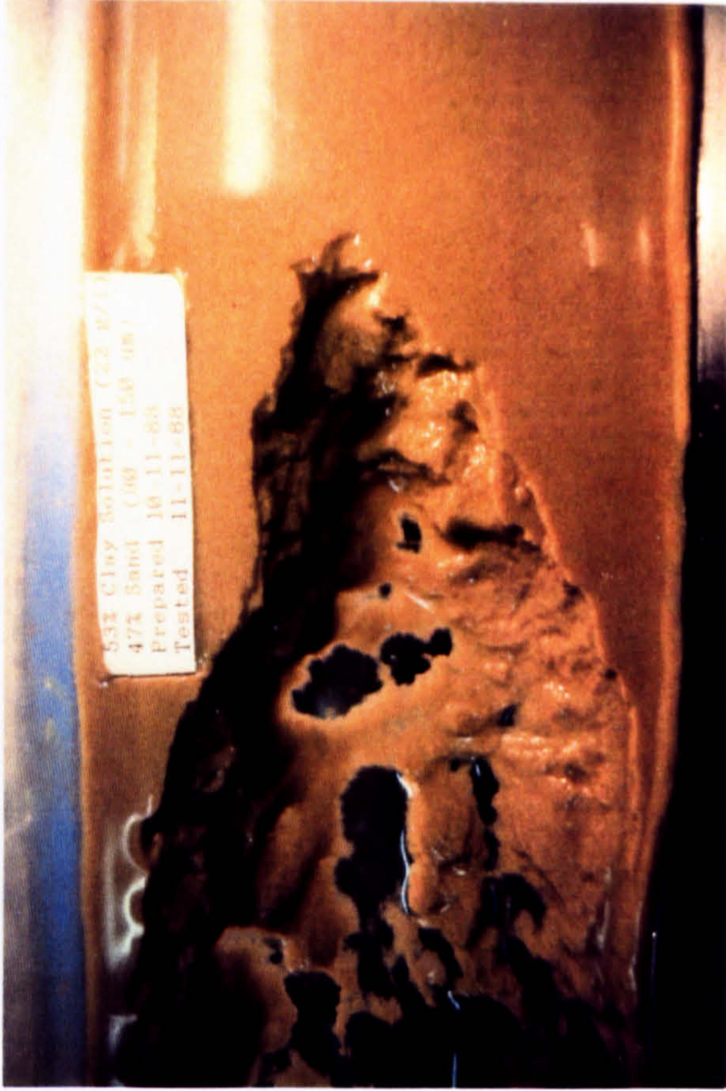
PLATE 10: Sediment bed after the collapse occurred Mixture: 53% Clay gel (22 g/l), 47% Sand (0.12mm)
