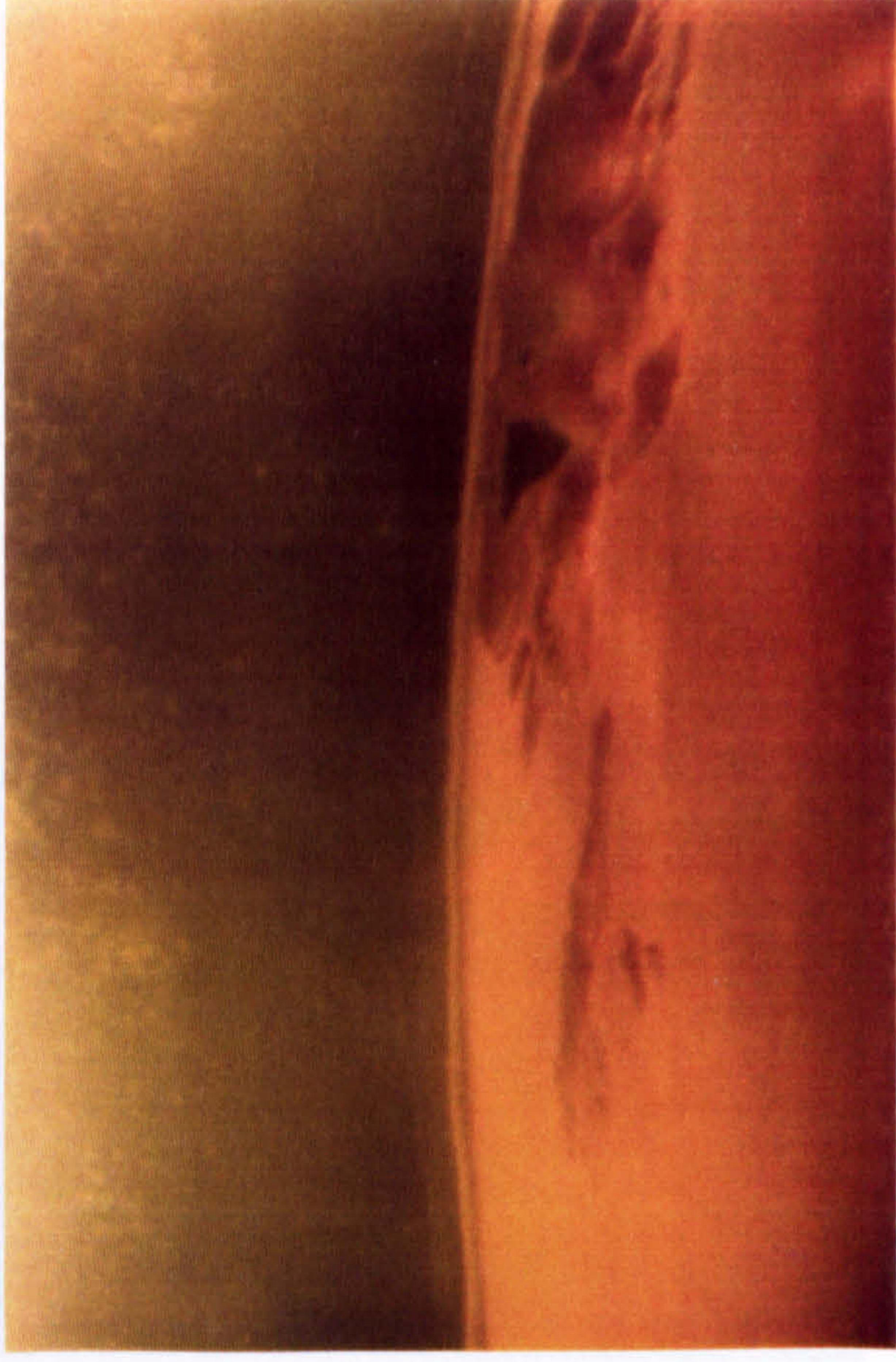
PLATE 7: Bed collapse, erosion progressing very rapidly ( \tau_{02} )
