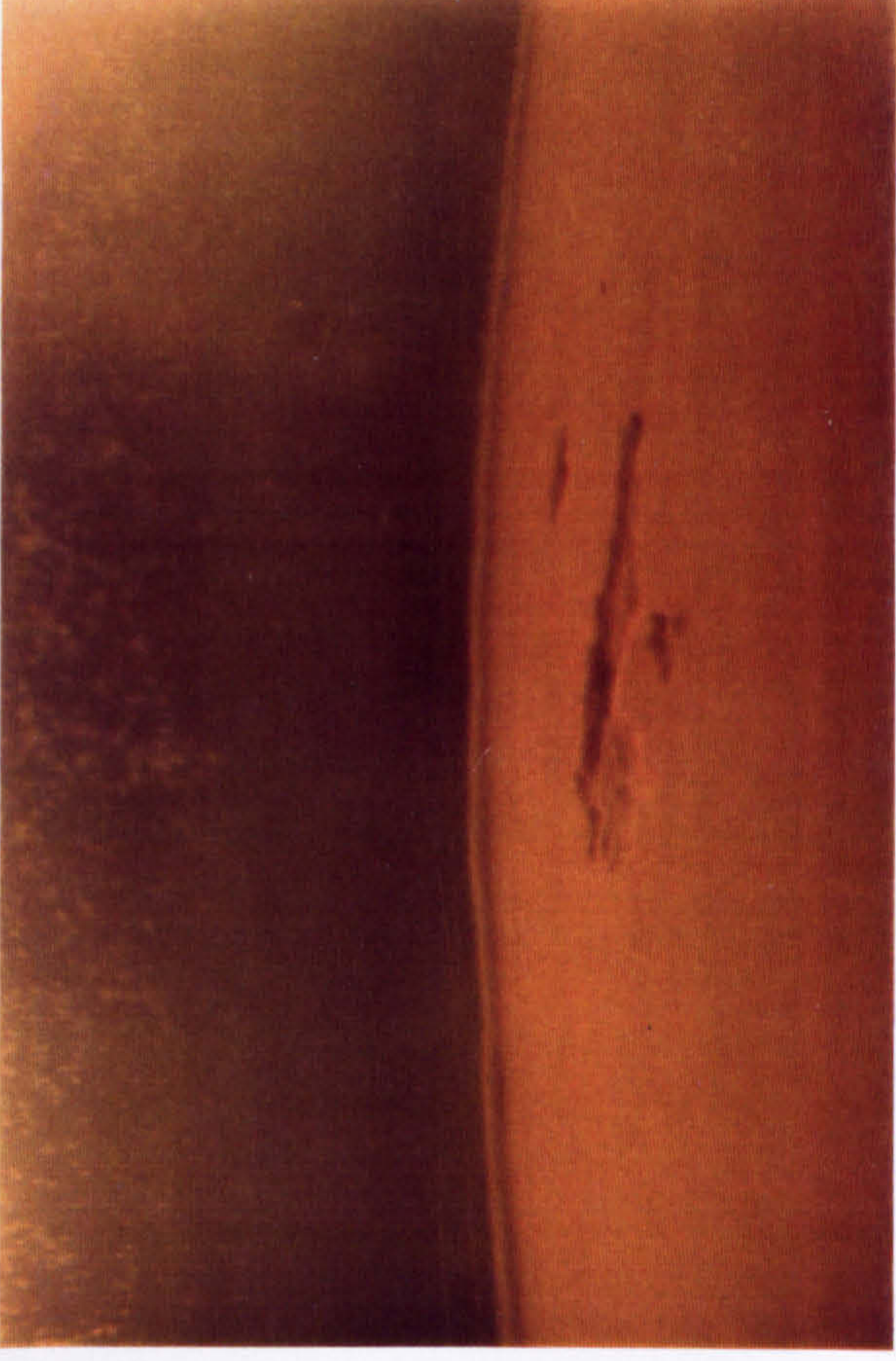
PLATE 6: First spots of erosion appearing on the bed surface ( \tau_{01} )
