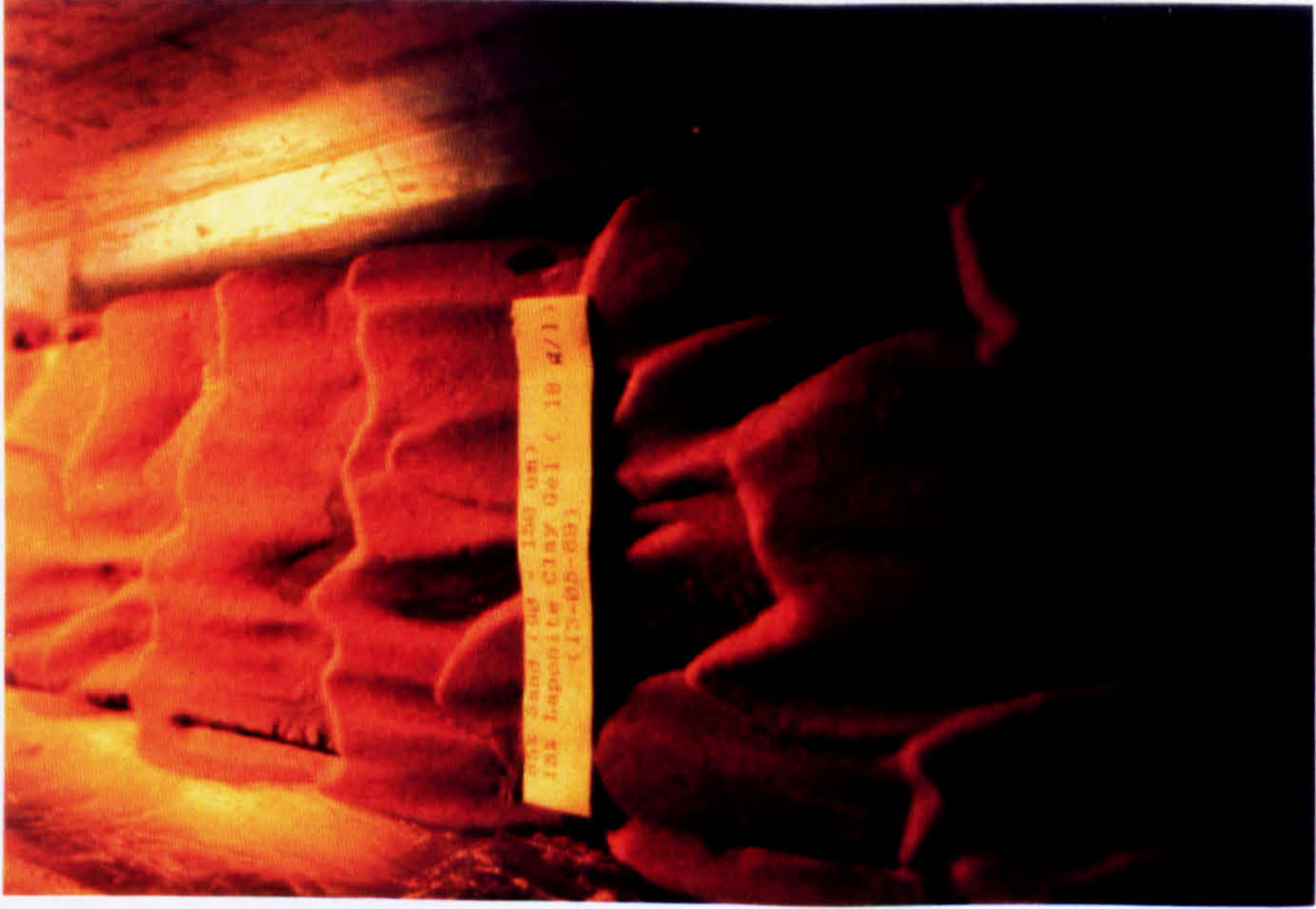
PLATE 8: Bed formation (85% sand ( d_{50}=0.12\text{mm} ) 15% clay gel (18 g/l))
