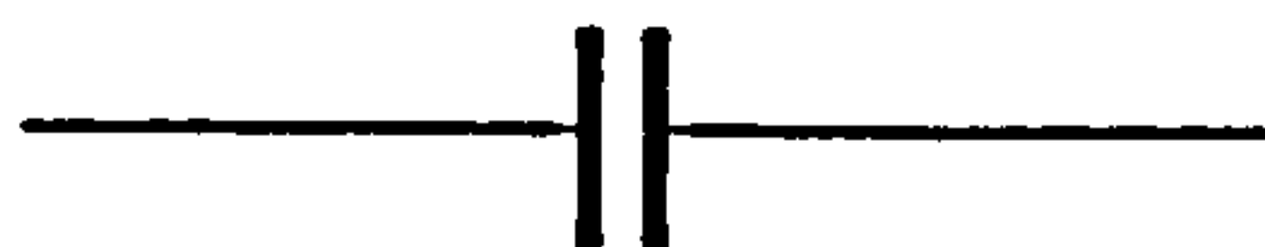
Fig 4.3. Equivalent circuit of an ideal polarised electrode
