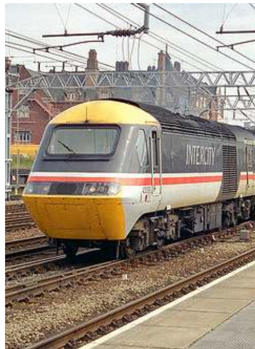
Figure 1.5. The Intercity 125 passenger train utilised a sandwich design for the driver’s cab [10].
