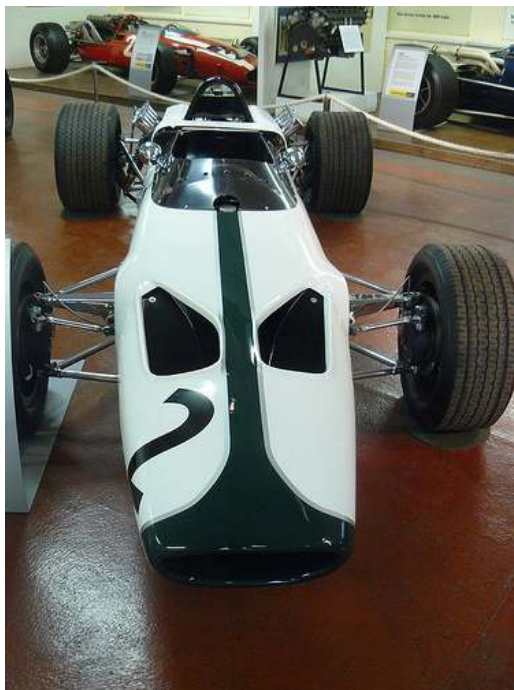
Figure 1.4. McLaren M2B, the first Formula 1 car to be raced that utilised a sandwich chassis [9].
