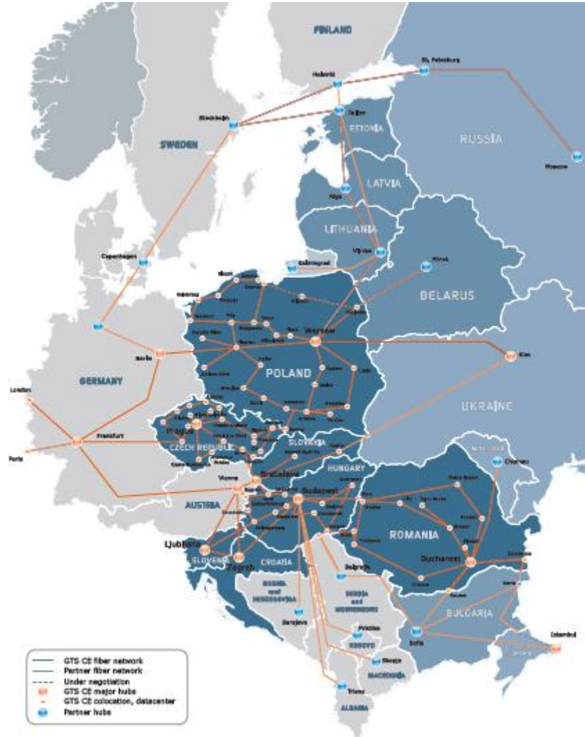
Figure A5.1: GTS European backbone network in Europe Source: GTS 2009
