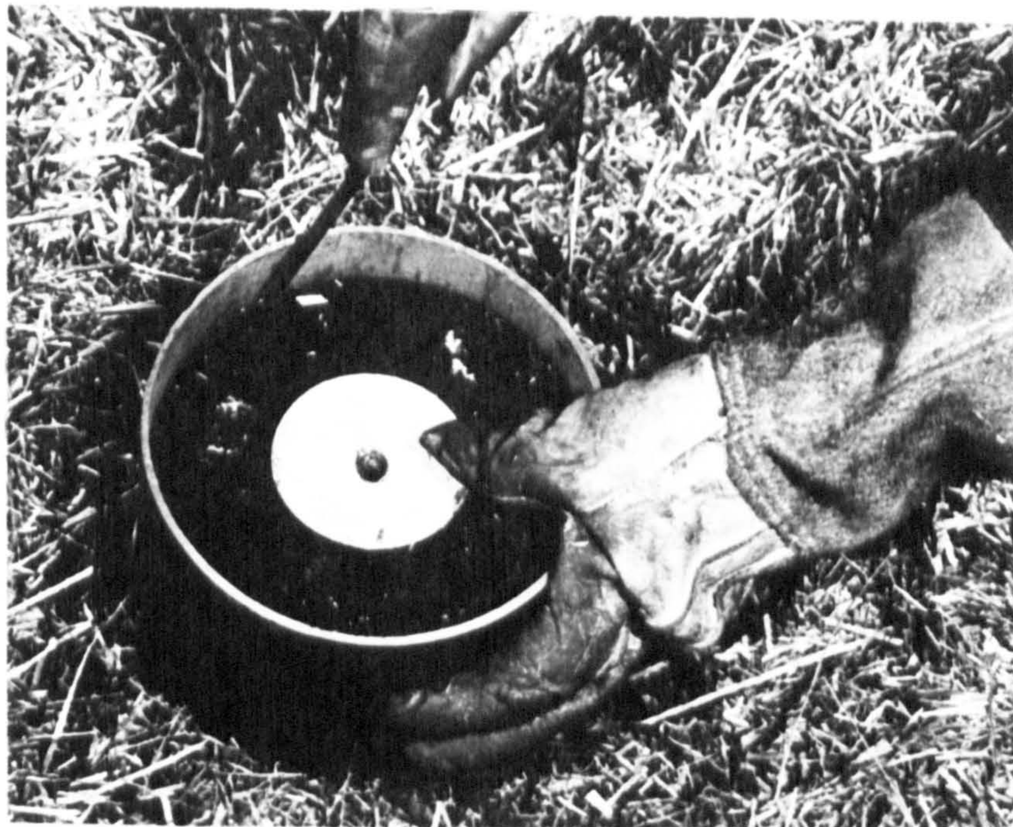
Fig.5.5/3 6 \frac{1}{4} " dia. Core Cutter in use at Glantlees. The piston inside the core cutter serves as a guide for the knife which is used to pre- cut the silage below the core cutting edge.
