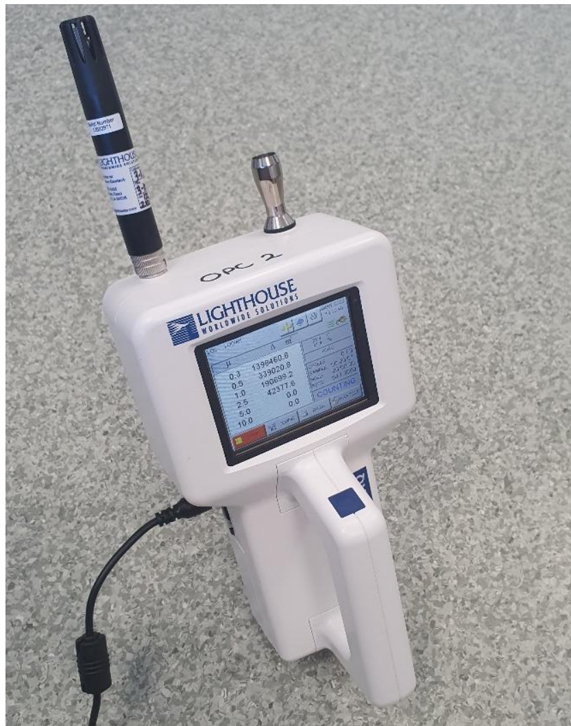
Figure 1.3. An optical particle counter.
