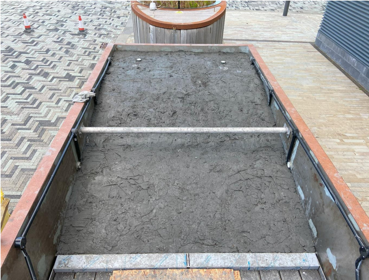
Figure 3.10: Photograph of the lysimeter slope immediately post-construction, illustrating the slope geometry.
