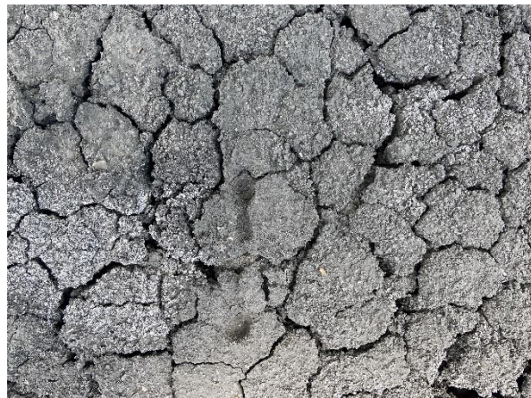
Figure 4.4: Time series of desiccation crack images showing the unstable aperture of the deep primary cracks within the Summer 2022 network after they first emerged in late May before later stabilising in mid-June.
