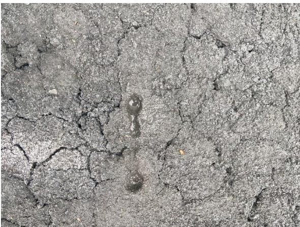
Figure 4.4: Time series of desiccation crack images showing the unstable aperture of the deep primary cracks within the Summer 2022 network after they first emerged in late May before later stabilising in mid-June.
