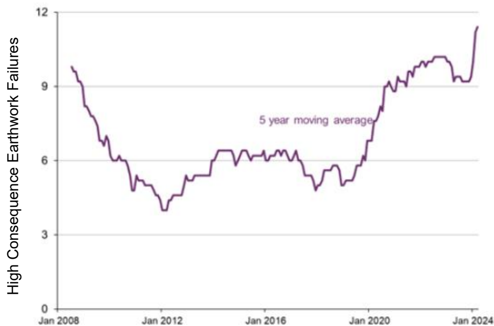
Figure 1.1: The number of high-consequence earthwork failures occurring within Network Rail's earthworks since the metric began in 2008 (from ORR, 2024)
