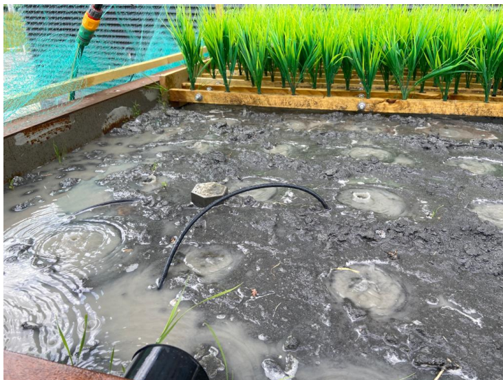
Figure 4.26: Image demonstrating the substantial ponding of rainwater in the crest (Side A photographed here) during E6 application due to its saturated state.
