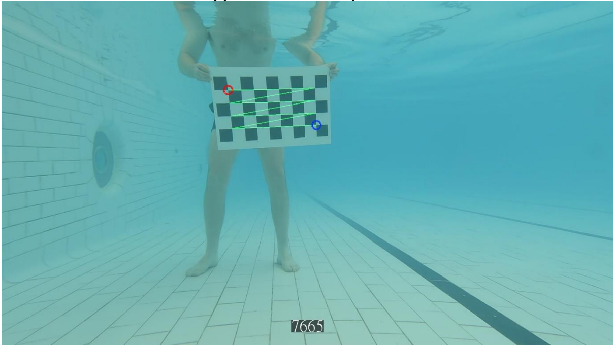
Figure S3.1 Example image from the stereo-video corner detection in the StereoMorph calibrateCameras function.
