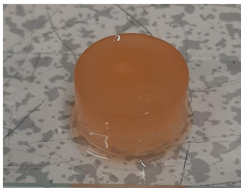
Figure 116. Image showing a slice of poly(thiopheneethanol) which is an orange gel structure.
