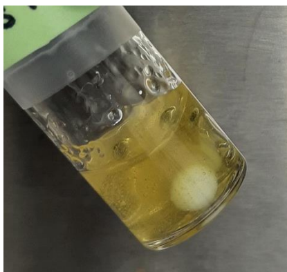
Figure 113. Image depicting the colour of PETE-S during the polymerisation reaction.
