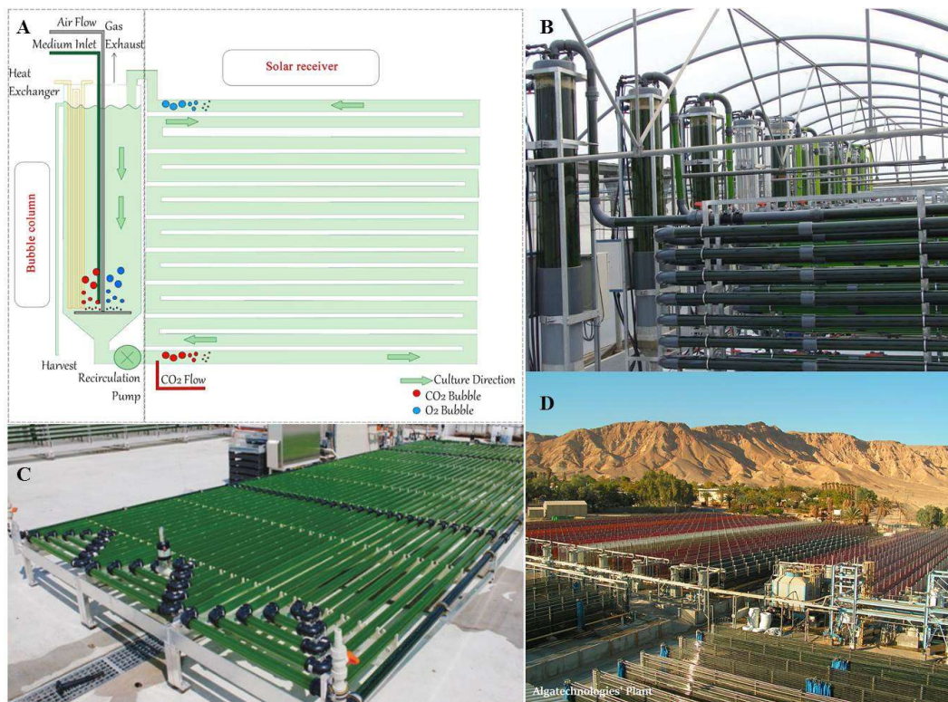
Figure 2.10: (A) a schematic of a tubular PBRs system, (B) a pilot-scale vertically stacked tubular photobioreactor in Almera, Spain (Fernández et al. , 2014), (C) a horizontal tubular photobioreactor at AlgaePARC, Wageningen UR, Netherlands (Placzek et al. , 2017) and (D) a commercial Haematococcus pluvialis production facility at Algatechnologies Ltd. in Kibbutz Ketura, Israel. (Photo courtesy of Solabia-Algatech Nutrition).
