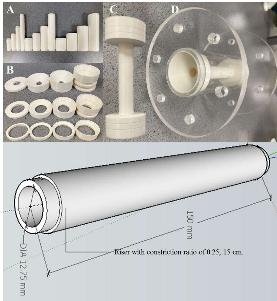
Figure 3.3: Side view of some of 51 variable modules of the foam riser, (A) variable lengths and constriction ratios, (B) angles and constriction ratios, (C) as desired, a combination of variable length and variable angle was constructed to form a type of riser and (D) the desired riser was then inserted into the transparent acrylic tube.
