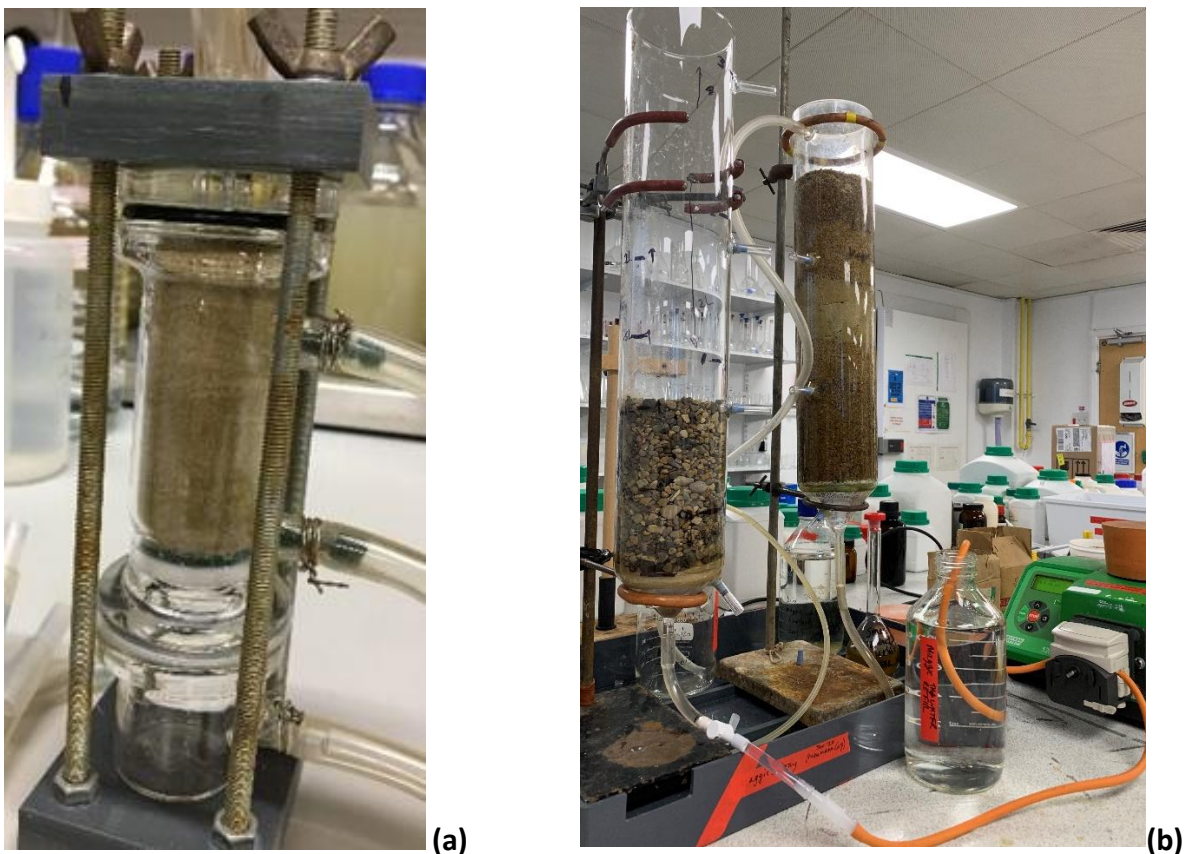
Figure 3. 4 (a) Small glass column packed with <2\ \mu\text{m} nontronite clay and high purity quartz sand (in a 1:50 ratio). (b) Open-topped large glass columns being packed with either pea gravel, coarse or medium sand above and below the clay and sand 'reactive layer'.
