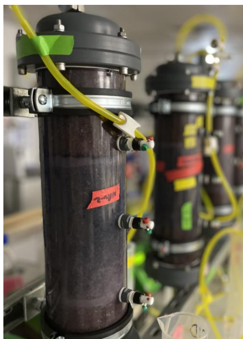
Figure 5. 6. Image of microbially-activated NAu-2 biological column, 20 days after inoculation. Not the very dark green which is characteristic of reduced nontronite clay.
