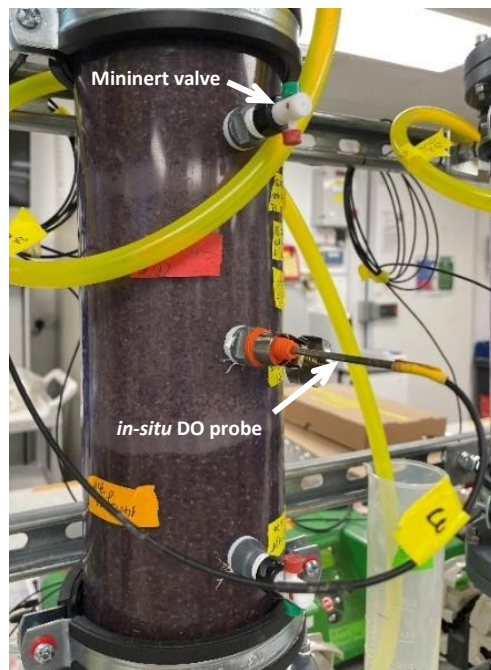
Figure 3. 10. An in-situ dissolved oxygen (DO) probe is sealed inside the central sampling port of large packed experimental column. A sub-seal bung and hose clip are used to form an airtight seal between the probe and the column sampling port.
