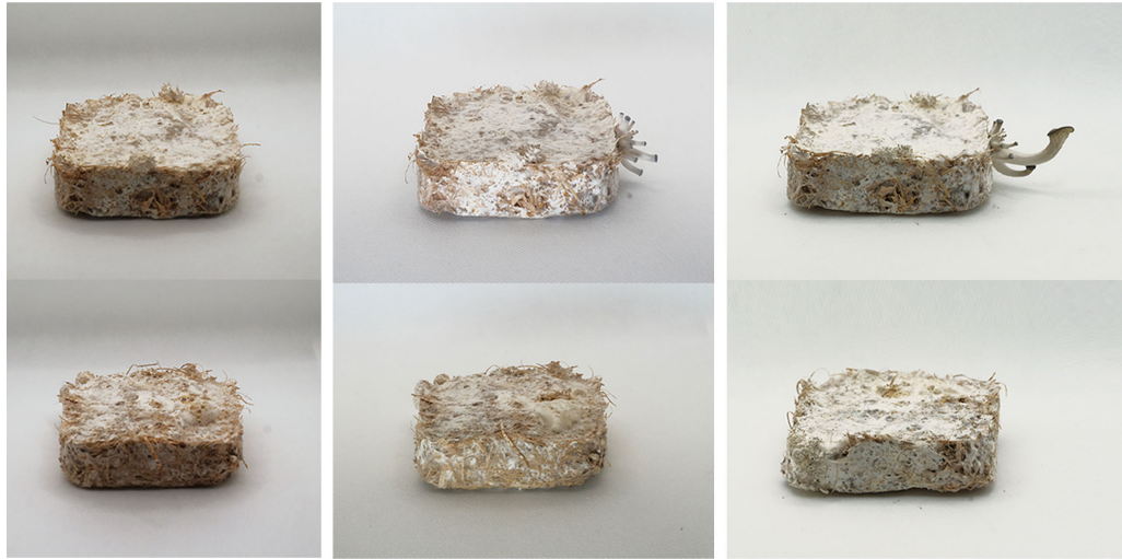
Figure 15 Mushroom curvature variations on days 21, 23 and 27 in flat-pack moulds correlated with humidity levels.
