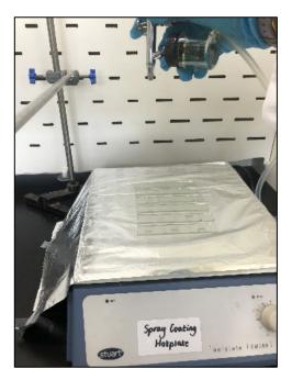
Figure 3.3: Manual spray coating of the  $TiO_2$  blocking layer via an airbrush and  $N_2$  carrier gas.
