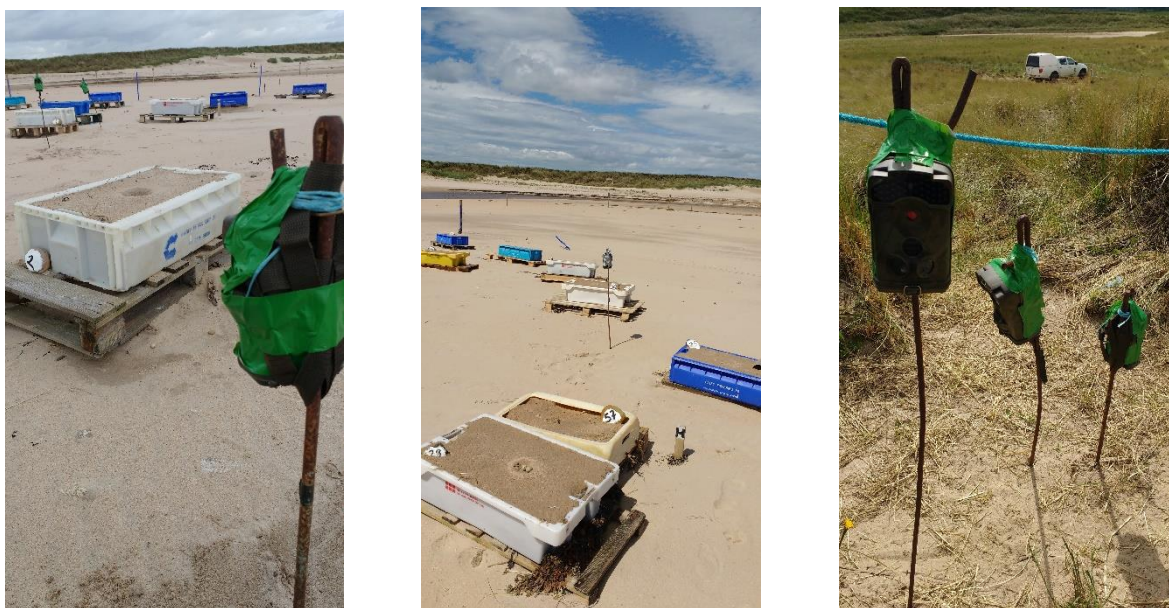
Figure 4.1. Examples of camera trap attachment to fencing pins. The use of fencing pins was necessary as scrapes at Long Nanny are raised on to fishing crates and pallets to provide protection from high tides. The first two images (left and centre) show cameras and fencing pins in place within the colony. Photographs and Placement of the traps was covered by a licence to disturb Schedule 1 Birds obtained from Natural England by (Ref: 2017-28158-SCI-SCI).
