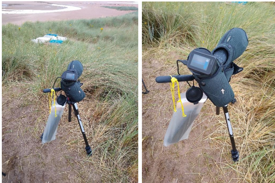
Figure 4.3. Illustration of digi-scope arrangement. A GoPro Hero 7 is attached to a Swarovski scope using a commercially available digi-scope attachment. To increase the battery life of the GoPro it was attached to a power bank using a USB cable. The power bank was held in a dry bag attached to the arm of the tripod mount.
