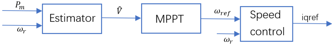
Figure 2.10 TCSE-based control diagram
