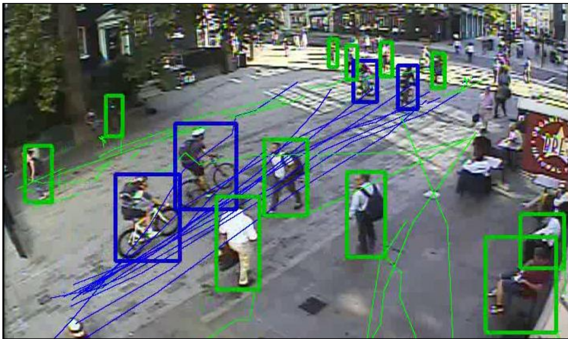
Figure 4.5. Multi-modal flows captured by Machine Vision cameras (Streets Systems, 2023)
