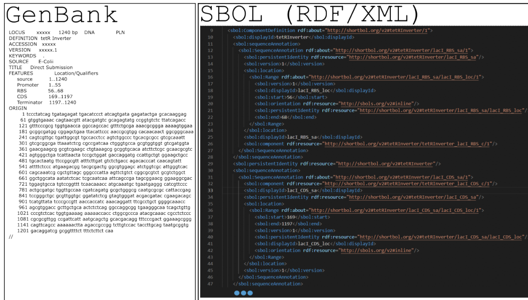
Figure 10: A GenBank file (Left) and SBOL encoded XML (Right) describing the same Gene (promoter, RBS, CDS and Terminator). The SBOL is cut off due to the large size of the document.
