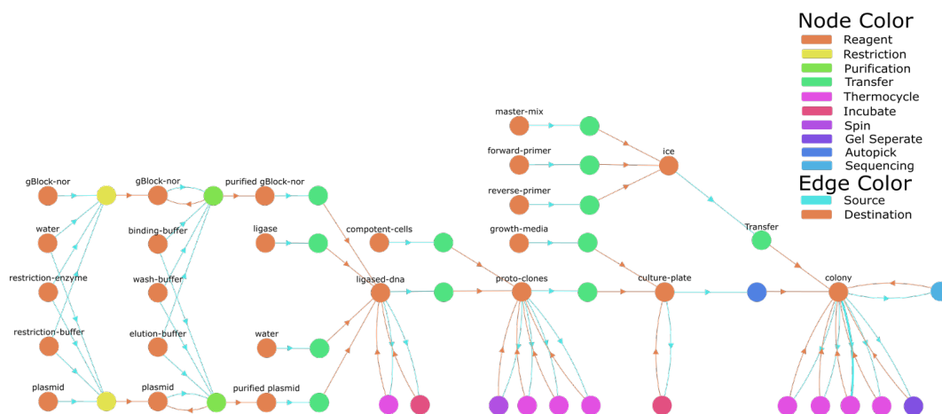
Figure 26: The NOR gate build protocol's input/output representation. Nodes represent physical entities such as reagents, and abstract actions such as transferring liquids and edges represent connections to sources and destinations.
