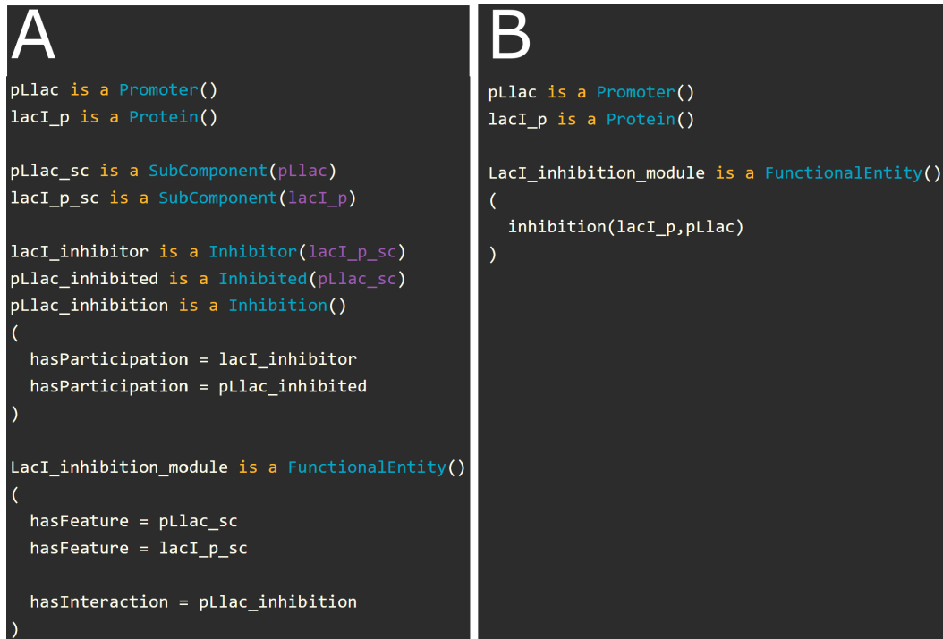
Figure 10: A comparison of the A: “Developer mode” and the B: “User mode” defining the same protein-promoter inhibition. The composite (inhibition) within the “User mode” is defined within another template as the context is required.
