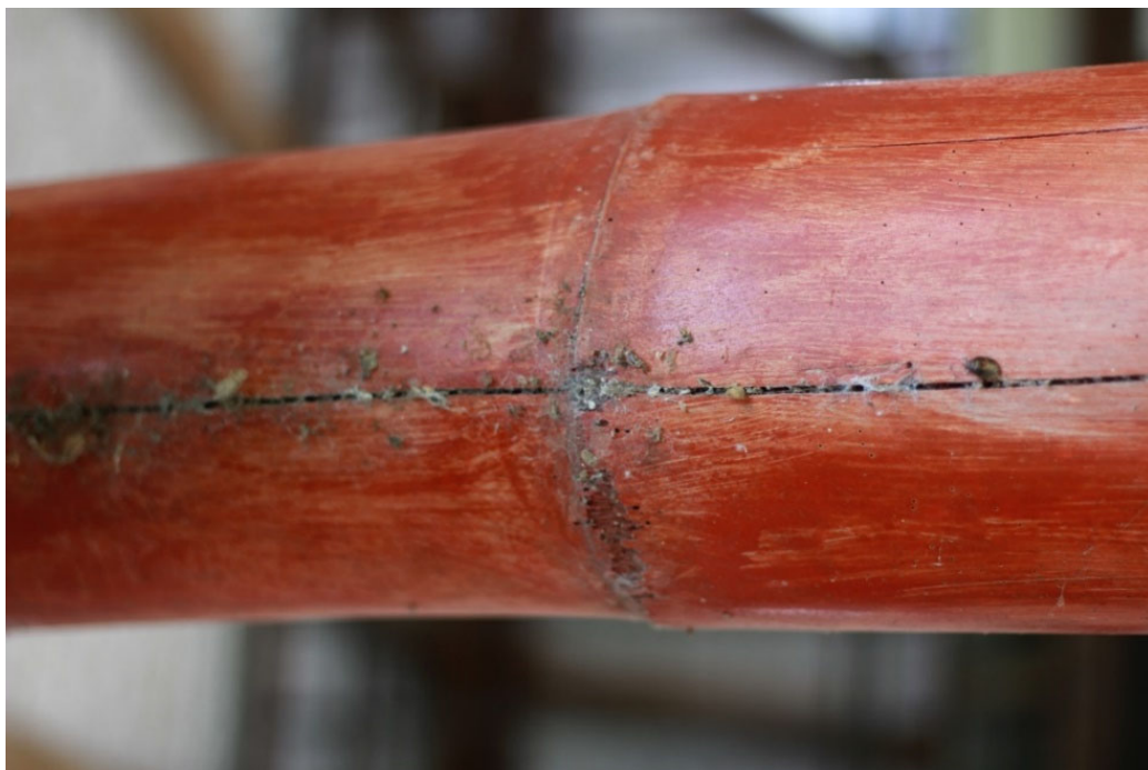
Figure 36: A crack in a painted piece of bamboo in which insects have penetrated inside. Photo by author, 2022.
