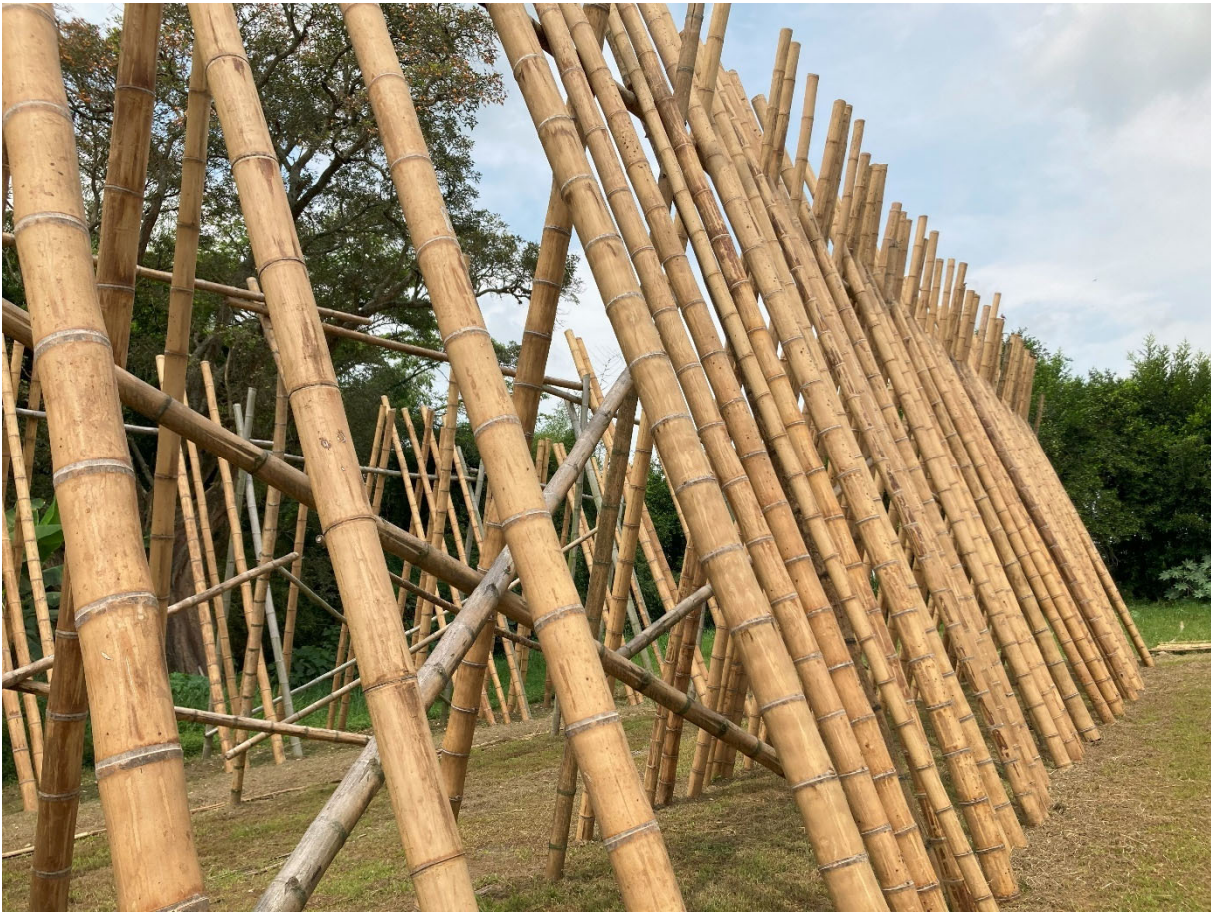
Figure 58: Air seasoning of bamboo poles drying in the open air and sun light. Photo by author, Ecobamboo bamboo treatment facility, outside Candelaria, Valle del Cauca, Colombia, 2022.
