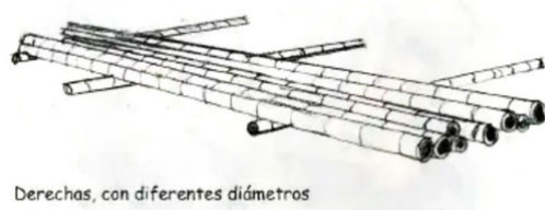
Figure 107: Visual grading applied to determine material availability: The process of sorting bamboo poles onsite for construction used during the Panama workshop, into straight poles (left), and poles with a single curvature (or bow) or more than one direction of curvature (right). Image reproduced from Stamm (2001, p. 34).
