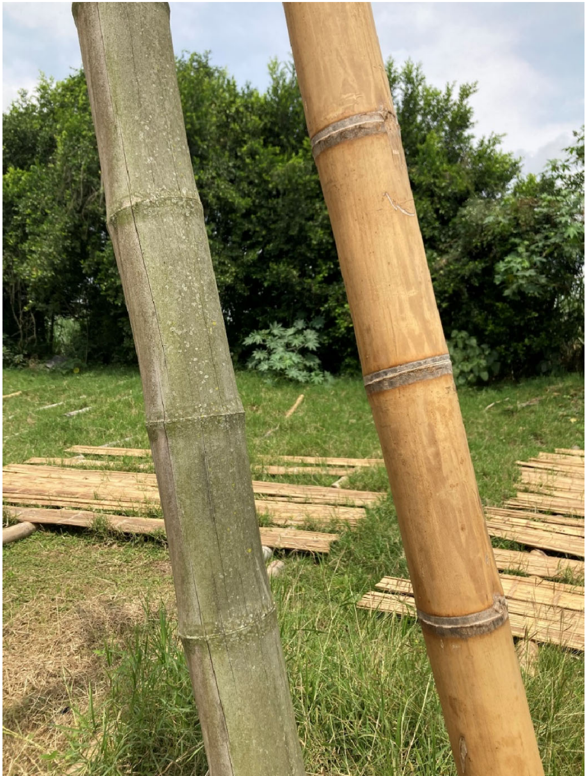
Figure 21: Two bamboo poles of the same species ( Guadua angustifolia ) from the same region. The left pole is used as a frame which has become grey, coarse and split because it has been exposed to the sun and the rain over a period of time and is used to support newly treated and drying bamboo poles (right). Photo by author, Ecobamboo bamboo treatment facility, outside Candelaria, Valle del Cauca, Colombia, 2022.
