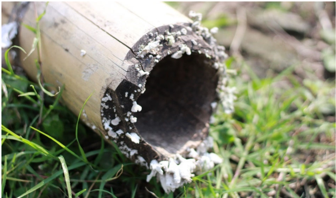
Figure 46: White-rot fungus, as a result of excess moisture. Photo by author, 2022.
