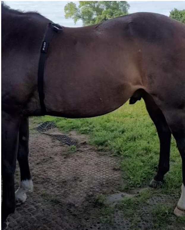
Figure 6.4 Placement of the Polar Equine Heart rate monitor using a Polar equine band.
