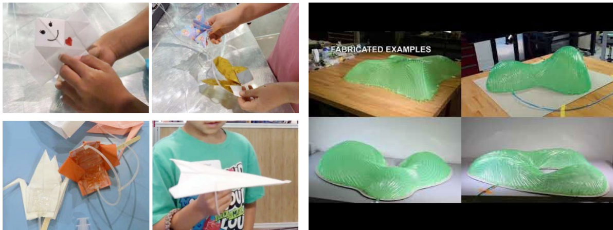
Figure 22: Examples of the use of pneumatics for actuators and shape-changing interfaces. On the left, the Sticky actuator [379], on the right, aeroMorph project [279].
