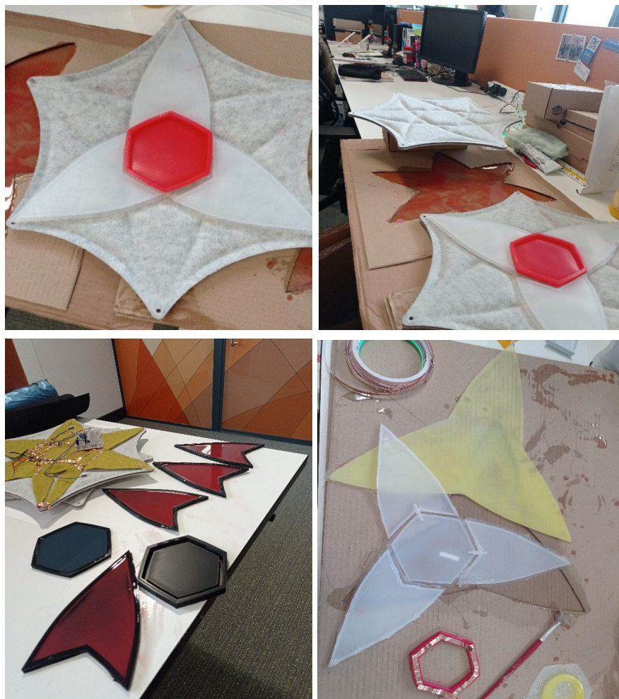
Figure 96: Combining silicone and thermochromic pigments
