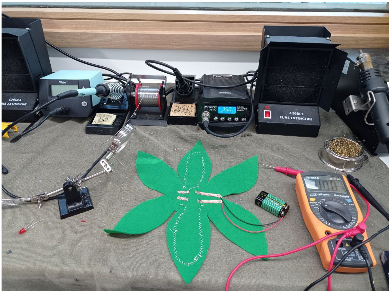
Figure 87: Creating a folding flower; The 'flapping crane' experiment tailored to my design case. Testing folding of a flower-shaped felt fabric using SMA wire (0.06HT) in a serial circuit made out of copper tape. The folding effect was tested using a 9Volt battery and at 13,5Voltage/ 0.45Amper current using an adjustable power supply machine.
