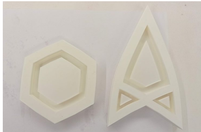
Figure 90: Designing and 3D-printing molds in different thicknesses to cast silicone to dry. Pouches were produced by gluing the silicone parts together using silicon. Initially produced silicone was too thick (the molds were too deep) and the sides were too narrow, resulting in insufficient attachment of silicone layers and air leaking.
