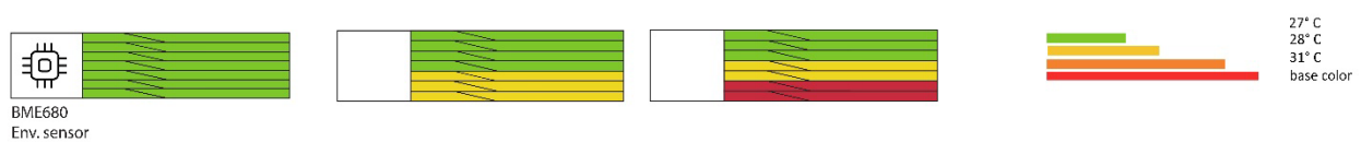
Figure 70: A concept of visualizing historic climatic data (24 hours of climatic timeseries) with layered thermochromic pigments (that have different temperature thresholds)
