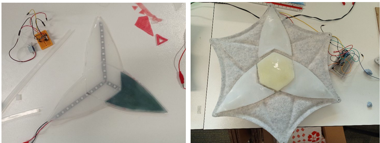
Figure 99: Attaching the LEDs on the back of the silicone pouches, and creating a final module that inflates and illuminates/changes color using the LEDs.
