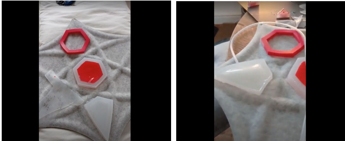
Figure 91: Testing inflation in silicone-made pouches and thermochromic change of thin silicone layers (colored with thermochromic pigments) when heated.
