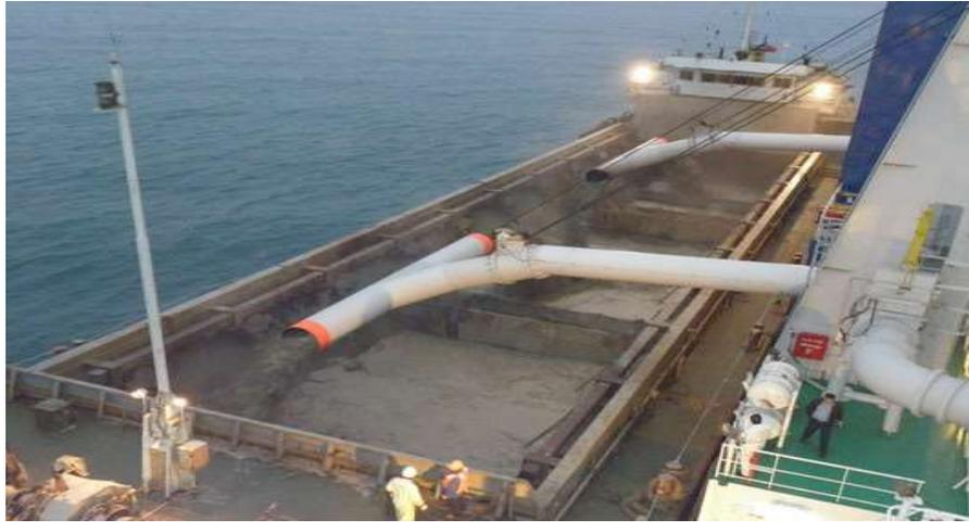
Figure 17. Side-by-side configuration of the dredging ship and the mud barge (Song Chang, 2017).
