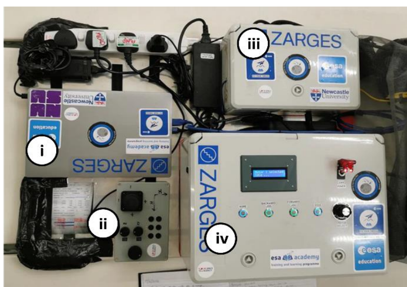
Figure 5.21 Gravityscope control baseplate with (i) laptop, (ii) microscope xy joystick and z dial controls, (iii) microscope power box and (iv) syringe pump power and control box.
