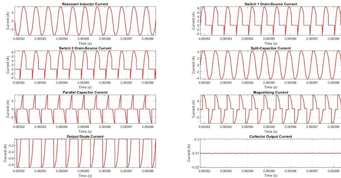
Fig.30: Full-Load Currents of the Series-Parallel Resonant Converter at 243V Line Voltage.
