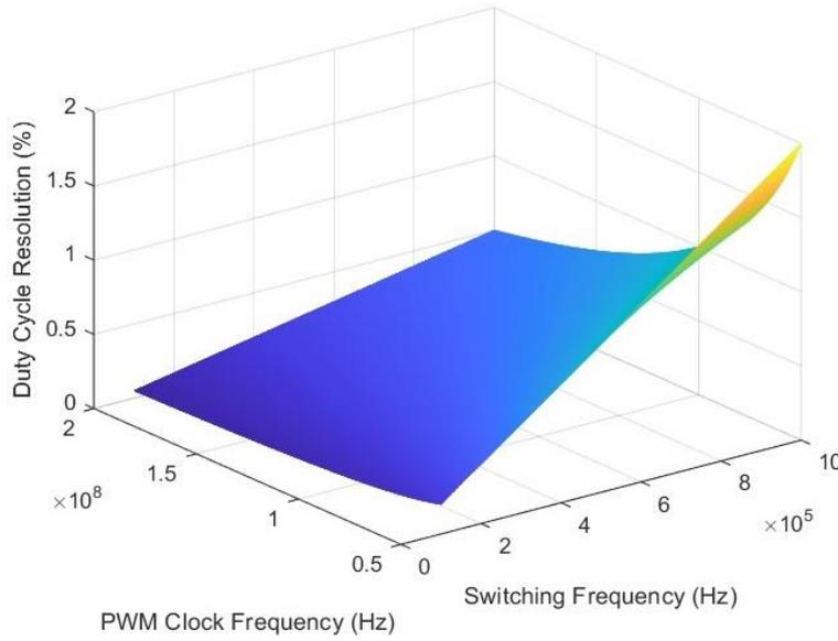
Fig.66: Visualization of Achievable Duty Cycle Resolution with Differing Switching Frequencies for Typical DSP CPU PWM Clock Rates.
