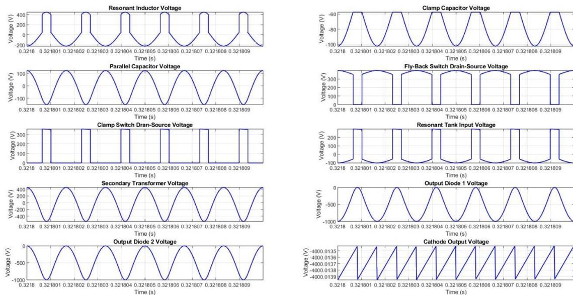
Fig.37: No-Load Resonant Fly-back Converter Voltage Waveforms with 297VDC Input Voltage at a Switching Frequency of 600kHz and ~22.4% Duty Cycle.
