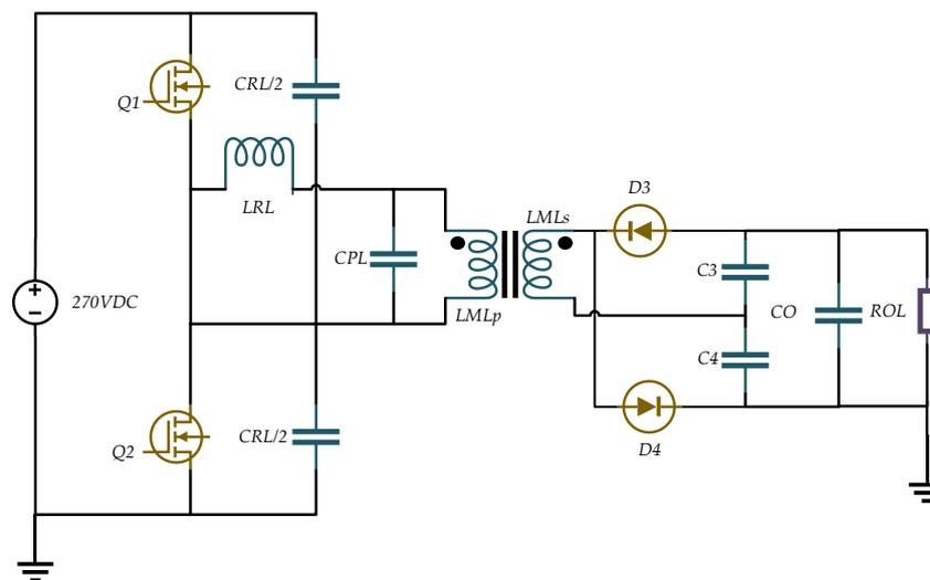
Fig.18: Series-Parallel Resonant LCC Regulator Topology.
