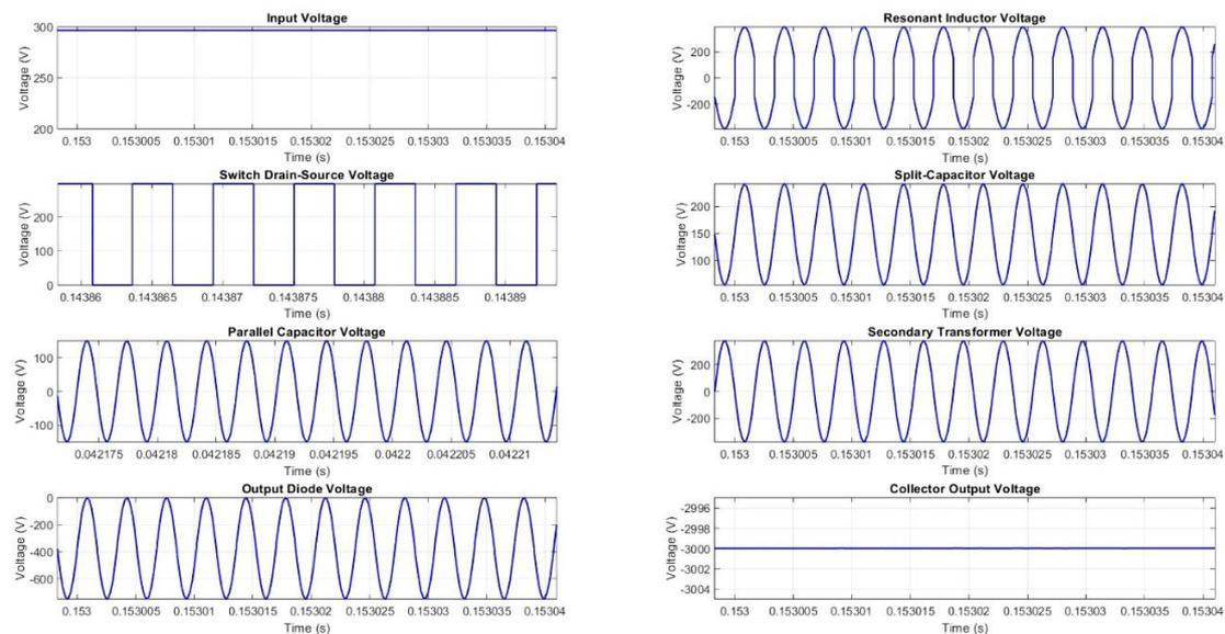
Fig.31: Full-Load Voltages of the Series-Parallel Resonant Converter at 297V Line Voltage.
