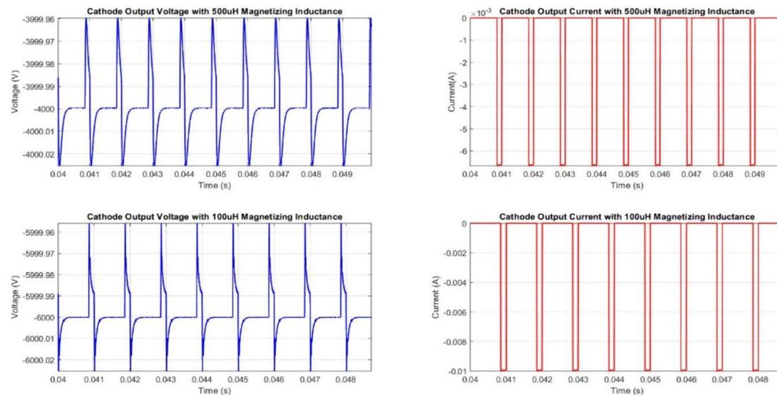
Fig.51: Transient Performance comparison of the Fixed-Frequency Active-Clamp Multi-Resonant Converter with Decreased Magnetizing Inductance.
