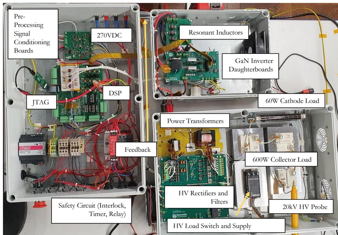
Fig.52: Experimental Test Rig Set-up Including Power Circuit and Digital Control Platform.
