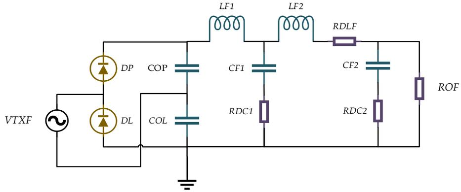
Fig.45: Second-Stage Filter with additional RC Filter Stage for Low-Noise Cathode.
