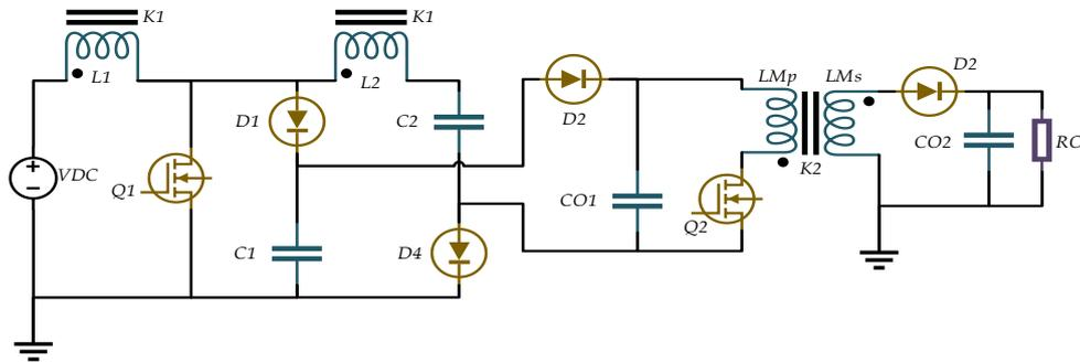
Fig.12: High-Gain Boost Pre-Regulator with a Single-Switch Fly-back Inverter Load.
