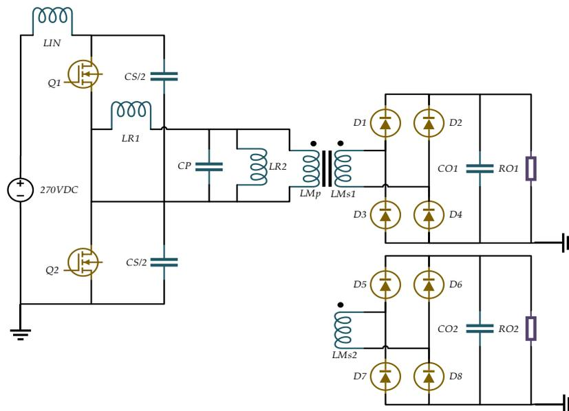
Fig.16: Current-Fed Four-Element Resonant Converter for Generation of a 500V Cathode Voltage with Wide Band-Gap Devices.
