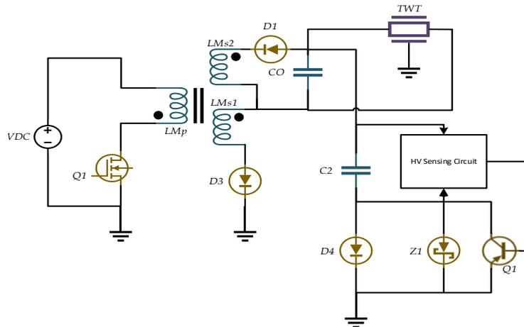
Fig.5: Secondary-Side Precision Linear BJT Regulator for Ultra Low-Noise TWT.
