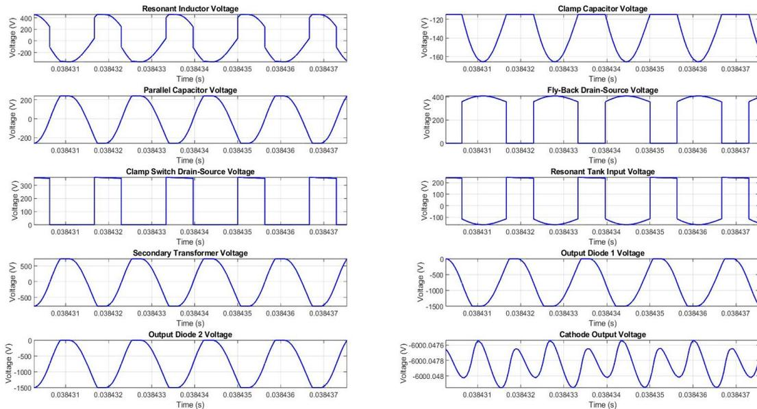
Fig.49: Full-Load LLCC Resonant Fly-back Converter Voltage Waveforms with 243VDC Input Voltage at a Switching Frequency of 600kHz and 35% Duty Cycle.
