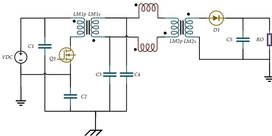
Fig. 14: Additional Isolation Transformer and Common-Mode Choke for Mitigation of Switched-Mode EMI Generation.
