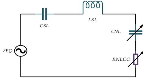
Fig.19: Capacitive Output Series-Parallel Model considering Transformer Non-Linearity.
