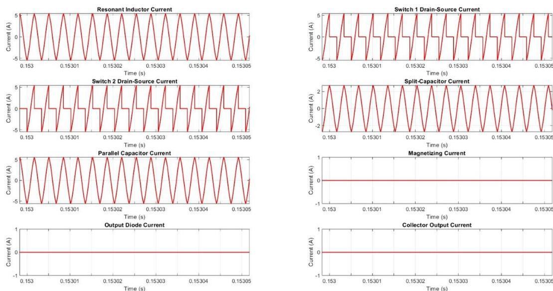
Fig.32: No-Load Currents of the Series-Parallel Resonant Converter at 297V Line Voltage.
