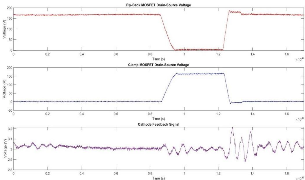
Fig.62: Cathode Feedback EMI Generation due to Hard-Switched Event at Fly-Back Switch Turn-Off.
