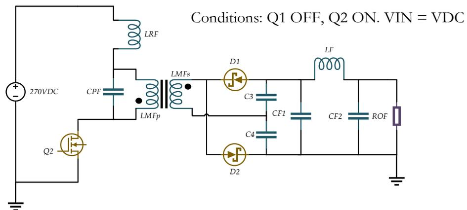
Fig.24: Parallel Resonance Stage of Multi-Resonant Fly-back Converter.
