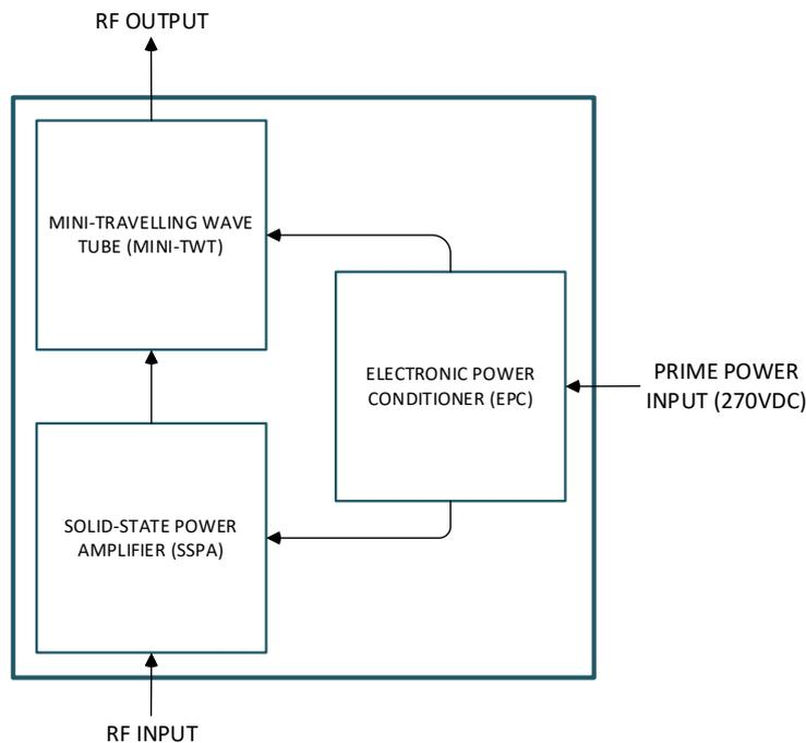
Fig.2: MPM Block Diagram Operating from 270VDC Prime Power DC Input.
