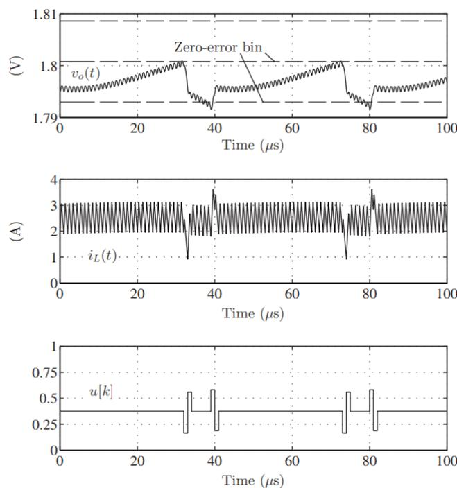
Fig.71: Limit Cycle Oscillation due to Coarse-Grained DPWM Duty Cycle Variations [133].
