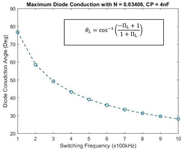
Fig.26: Graphical Representation of Diode Conduction Angle at Designed Transformer Characteristics with Simple Duty Cycle Modifications for Series-Parallel Resonant State.
