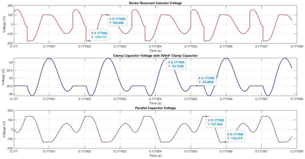
Fig.58: Relationship between Resonant Inductor, Clamp and Parallel Capacitor Voltages during Sub-Resonance Operation.
