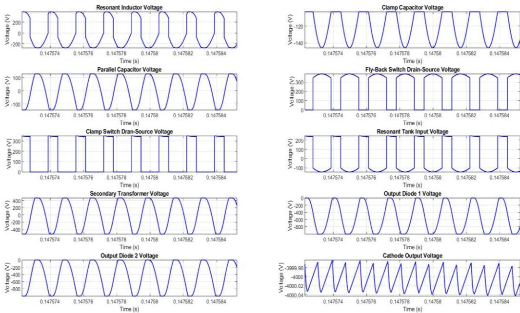
Fig.35: Full-Load Resonant Fly-back Converter Voltage Waveforms with 243VDC Input Voltage at a Switching Frequency of 600kHz and  $\sim 35\%$  Duty Cycle.
