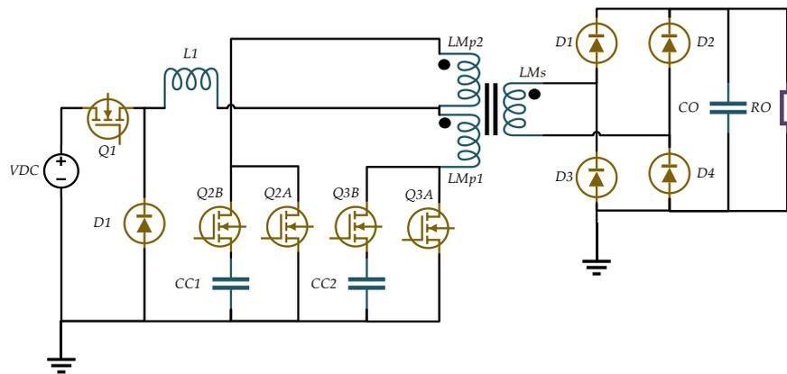
Fig.10: Buck Regulator Current-Fed Active-Clamped Push-Pull Converter.
