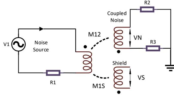
Fig.76: Coupled Noise due to Large Inductive Coupling Loop Areas.
