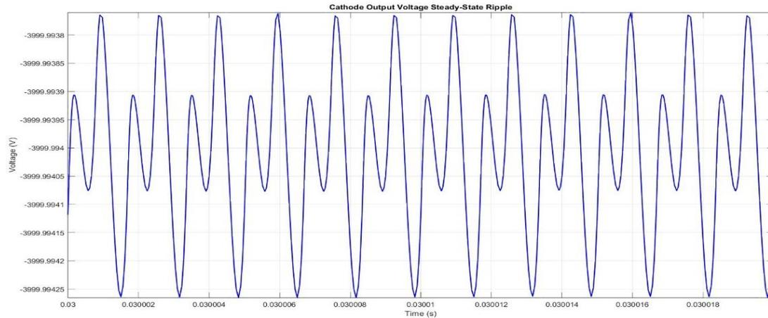
Fig.47: AC-Voltage Cathode Variation at Steady-State of approximately 500 $\mu$ V.
