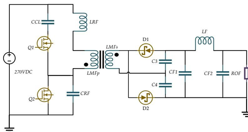
Fig.22: Active Clamp Fly-back Converter with Lumped Resonant Capacitance.
