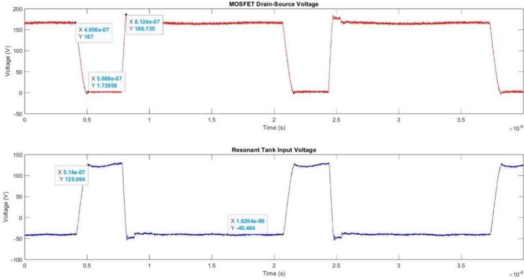
Fig.55: Drain-Source and Resonant Tank Input Voltages of the Multi-Resonant Fly-back.
