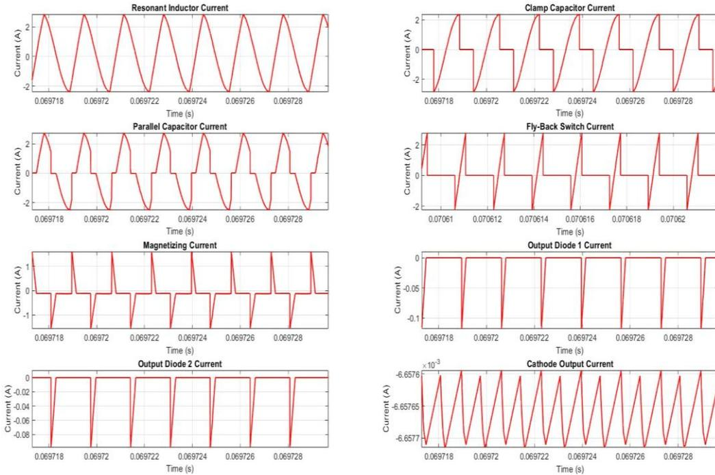
Fig.36: Full-Load Resonant Fly-back Converter Current Waveforms with 243VDC Input Voltage at a Switching Frequency of 600kHz and ~35% Duty Cycle.
