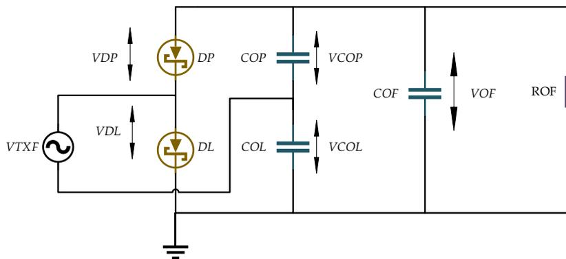
Fig.28: Development of an Average Cathode Voltage through Modulation of Individual State Capacitor Voltage Levels in a Full-Bridge Voltage Doubler Circuit.
