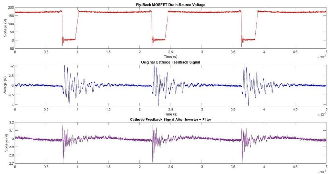
Fig.61: High Frequency Oscillations in Cathode Electrode Feedback Path.
