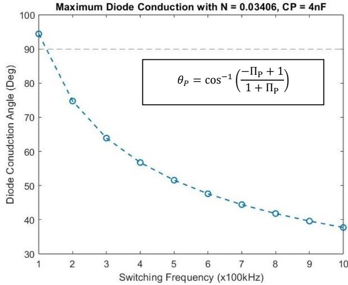
Fig.27: Graphical Representation of Diode Conduction Angle at Designed Transformer Characteristics with Simple Duty Cycle Modifications for Parallel Resonant State.
