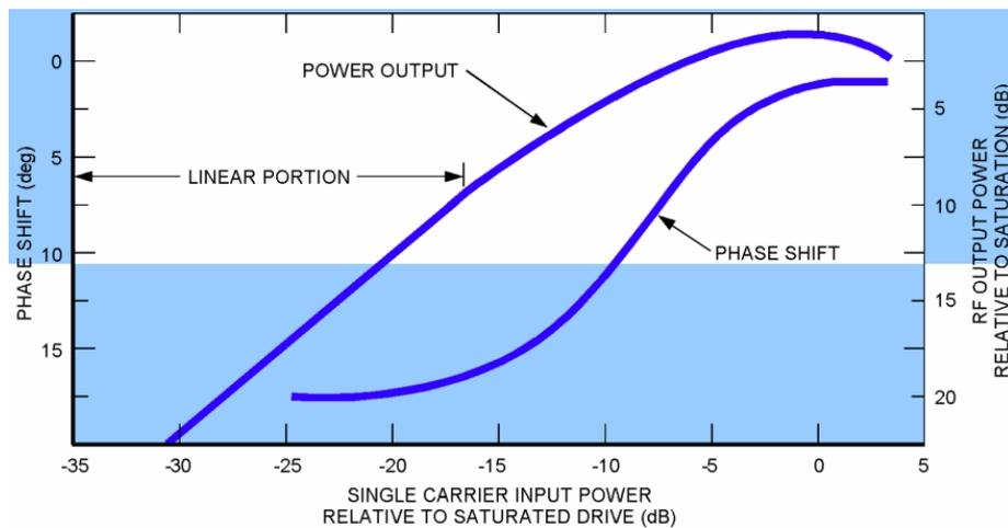
Fig.3: Power Output and Phase Shift as a function of RF Input Power showing the Linear and Saturated Amplification Points [27].
