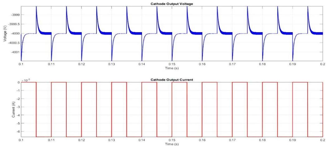
Fig.39: Low PRF Regime of 100Hz with a Duty Ratio of 50% with Voltage Mode Control.
