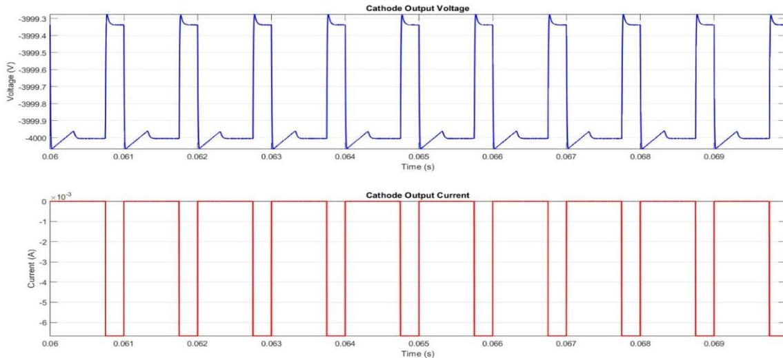
Fig.44: Low/Moderate PRF Regime of 1kHz with a Duty Ratio of 25% with ACMC and Current Sense Amplifier and Series Damped Pi-Filter.
