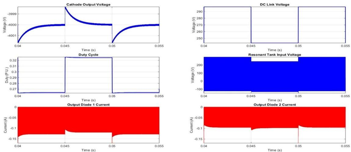
Fig.42: Transient Response during a 243-297V Input 100Hz Transient Event with VMC.
