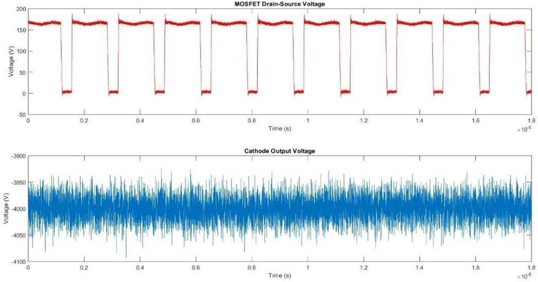
Fig.56: -4kVDC Cathode Output Voltage at 602kHz Switching Frequency at 22.4% Duty.
