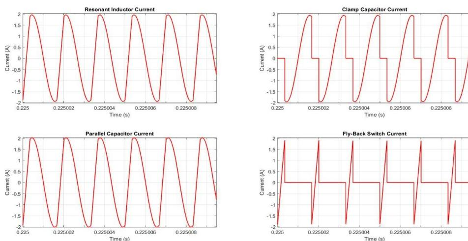
Fig.38: No-Load Resonant Fly-back Converter Current Waveforms with 297VDC Input Voltage at a Switching Frequency of 600kHz and ~22.4% Duty Cycle.
