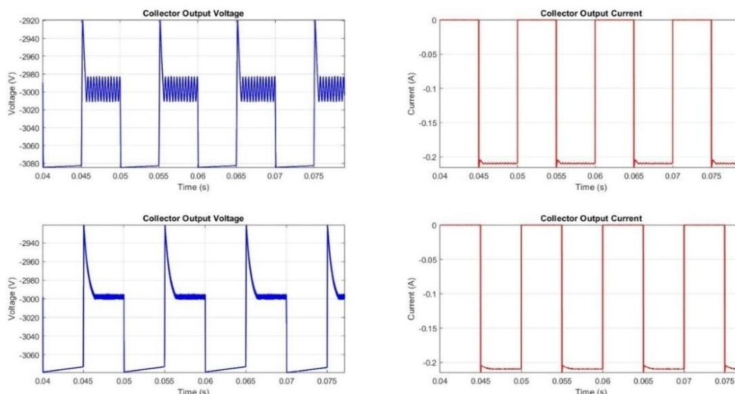
Fig.33: Instability of Collector EPC without (top left, right) and with (bottom left, bottom right) Sub Resonance Protection.
