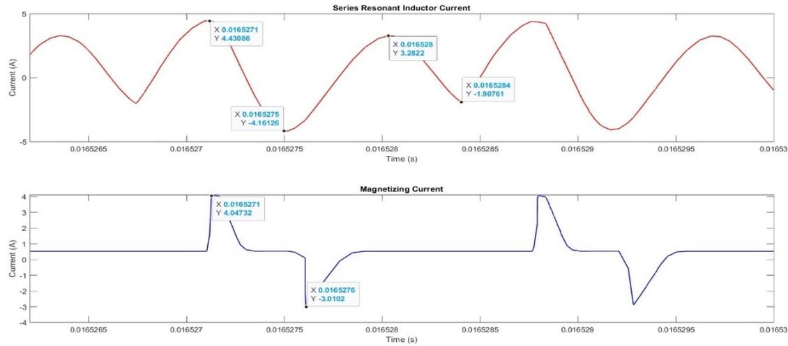
Fig.60: Current-Sharing Relationship between Series Resonant and Magnetizing Inductances.
