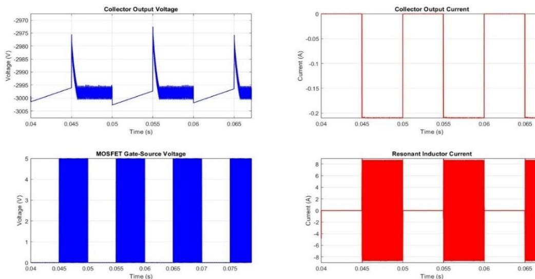
Fig.34: Simple Implementation of PRF Information to Reduce Transient Voltage Deviation within the Collector Electrode.
