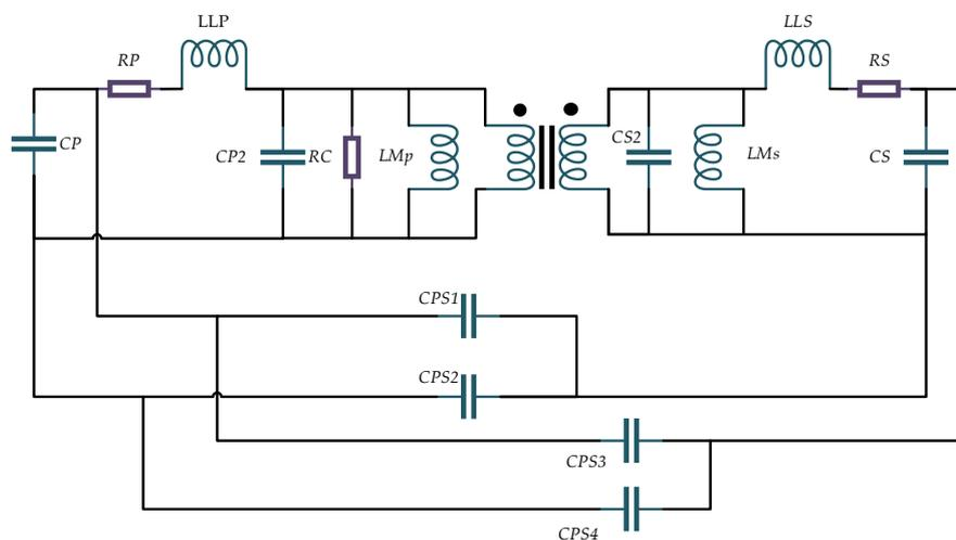
Fig.13: Transformer Model Including Common-Mode Capacitive Effects.
