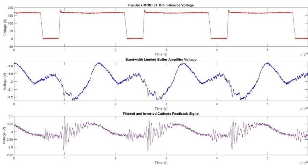
Fig.63: Filtered and Inverted Cathode Feedback Signal during Hard-Switching Event with Limited Bandwidth Buffer Operational Amplifier.
