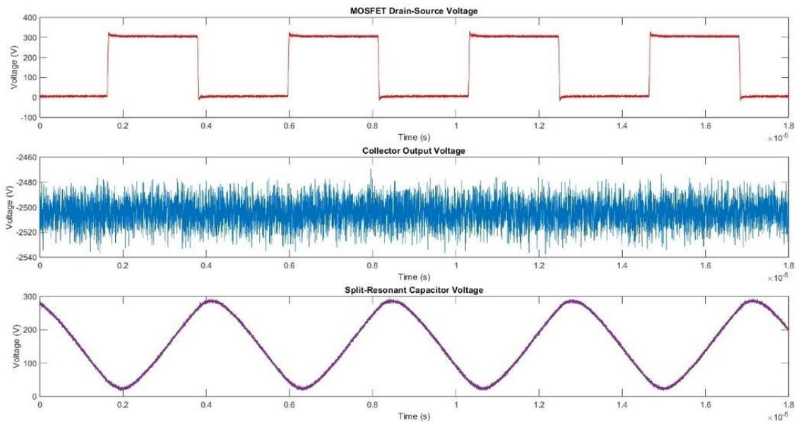
Fig.53: MOSFET Drain-Source and Split-Resonant Capacitor Switching Voltages with 297VDC Line Voltage.
