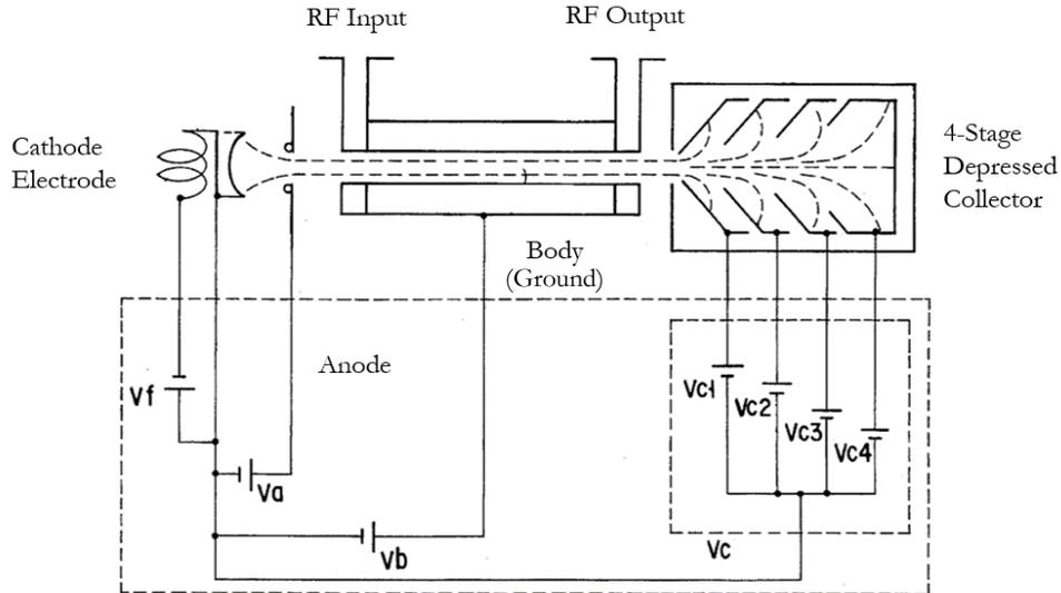
Fig.1: TWT Microwave Amplifier with Four-Stage Depressed Collector Configuration [8].
