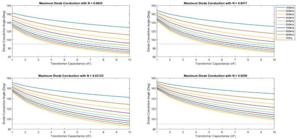
Fig.21: Required Diode Conduction Angles with Different Transformer Turns Ratios and Switching Frequencies for Differing Transformer Parasitic Capacitances with Load Resistance of 15K $\Omega$ .
