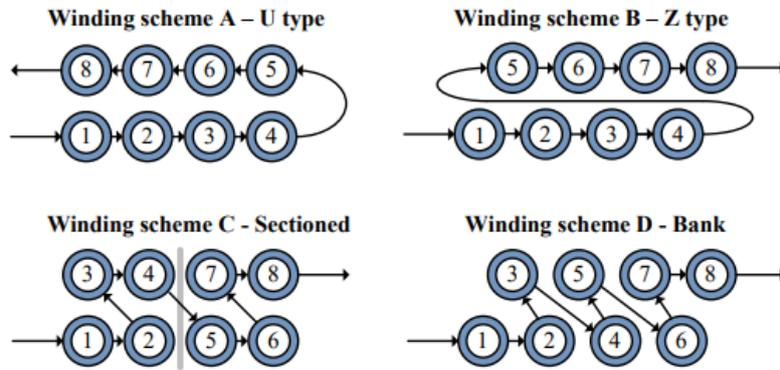
Fig.75: Commonly Implemented Transformer Winding Techniques [150].
