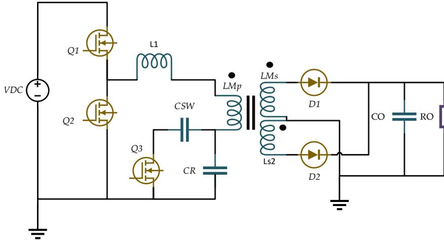
Fig.8: Fixed-Frequency Switched Capacitor Multi-Resonant SRC Converter.
