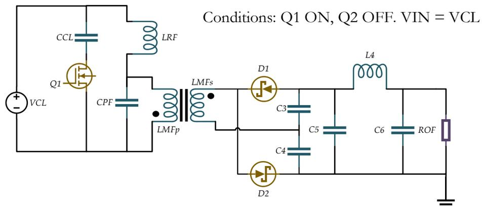
Fig.25: Series-Parallel Resonance Stage of Multi-Resonant Fly-back Converter.
