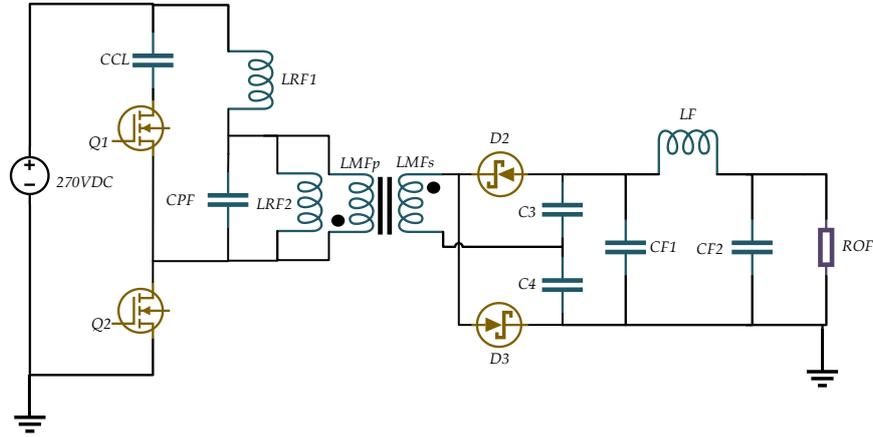
Fig.48: Proposed Four-Element Multi-Resonant Active-Clamped Fly-Back Converter Topology.
