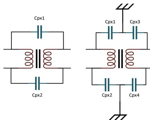
Fig.77: Inclusion of a Faraday Shield for Reducing Capacitive Coupling of Noise Voltage.
