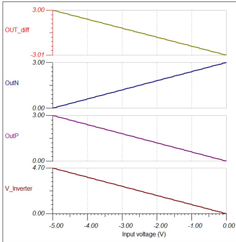
Fig.68: FDA Output Signals for a 0-5VDC Cathode Feedback Voltage.
