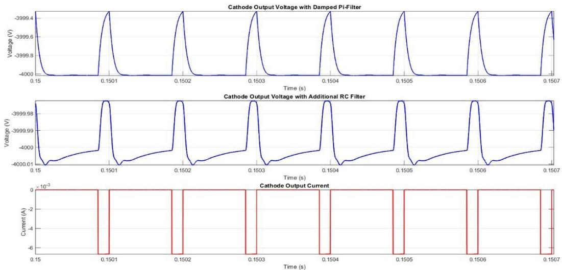
Fig.46: Comparison of Pi-Filter Alone and Additional R-C Filtering Techniques for Achieving Ultra-Low-Noise Cathode Electrode Voltages.
