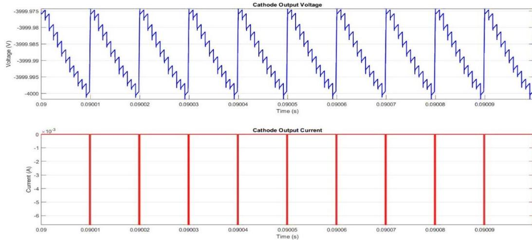
Fig.41: High PRF Regime of 100kHz with a Duty Ratio of 2% with Voltage Mode Controller.
