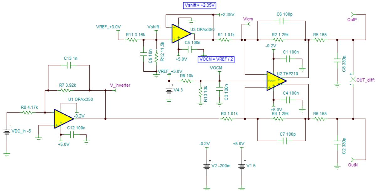
Fig.67: Utilizing a Fully Differential Amplifier to Translate a Single-Ended Source to an Equivalent Differential Signal for 16-bit Sampling.
