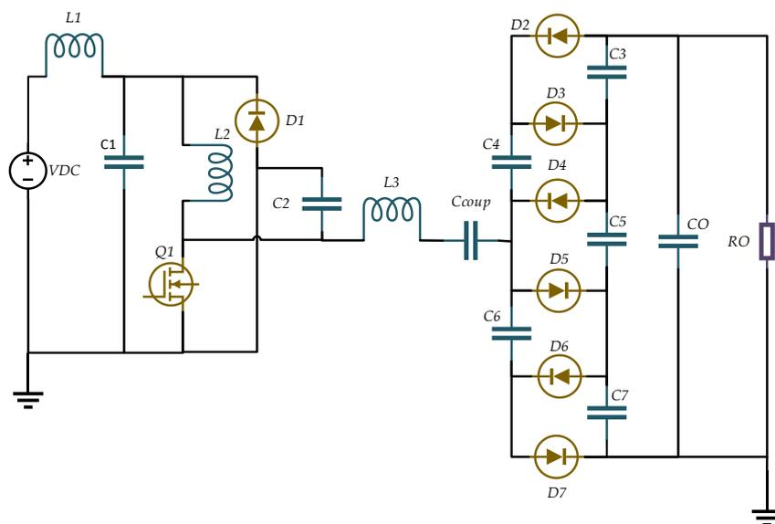
Fig.15: Capacitive Coupled EPC with Diode-Capacitor Chain Multiplier Circuit.
