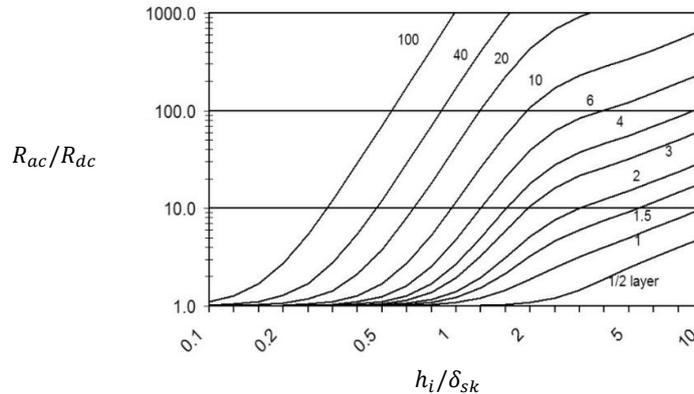
Fig.73: Normalized Dowell's Curves for AC/DC Winding Resistance with Differing Winding Configurations [147].
