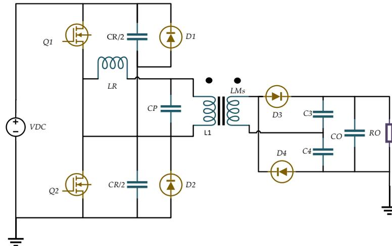
Fig.9: Diode-Clamped Split-Capacitor Resonant Converter for Long-Pulse Applications.
