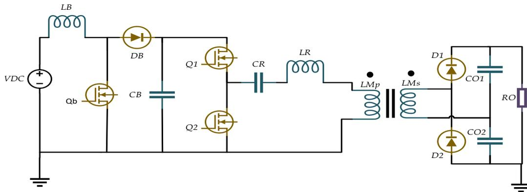
Fig.11: 300kHz Boost Pre-Regulator Stage with SRC Resonant Main Inverter.
