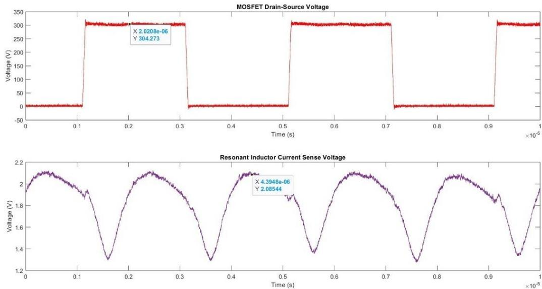
Fig.54: MOSFET Drain-Source Voltage and Series Resonant Inductor Current with 297VDC Line Voltage.
