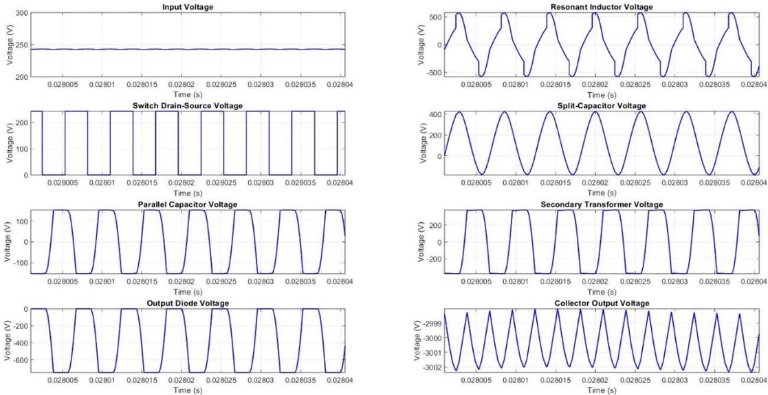
Fig.29: – Full-Load Voltages of the Series-Parallel Resonant Converter at 243V Line Voltage.
