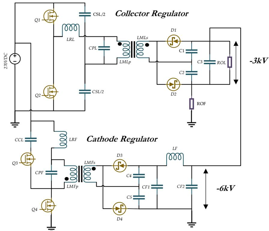
Fig.17: Proposed Novel Hybrid Fully Controllable EPC Topology for an MPM.
