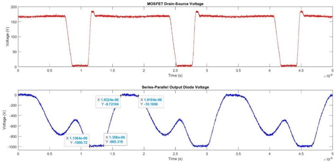
Fig.57: 1MHz Oscillating Series-Parallel Output Diode Voltage at 602kHz with 125VDC Line Voltage Indicating Diode Conduction Times during each state.
