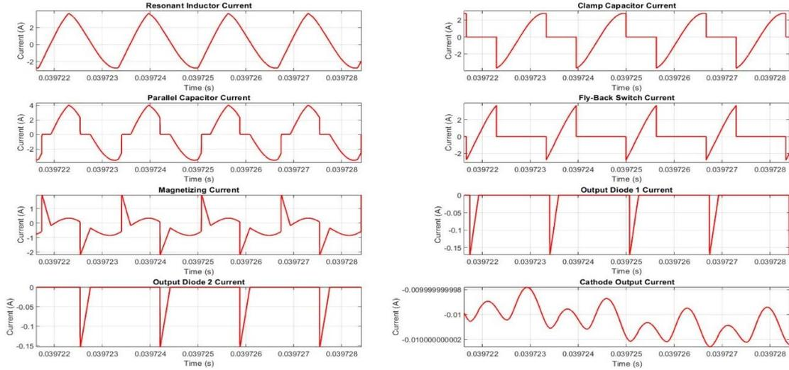
Fig.50: Full-Load Modified LLC Resonant Fly-back Converter Current Waveforms with 243VDC Input Voltage at a Switching Frequency of 600kHz and 35% Duty Cycle.
