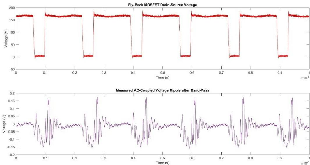
Fig65: AC Voltage Measurements within Cathode Utilizing Proposed AC-Coupled Circuit.
