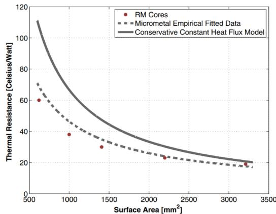
Fig.72: RM Core Thermal Resistances for Varying Surface Core Areas [140].
