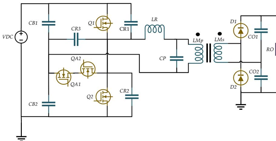
Fig.7: T-Type Converter with Bi-Directional Switching Cell for Asymmetrical Duty Control.
