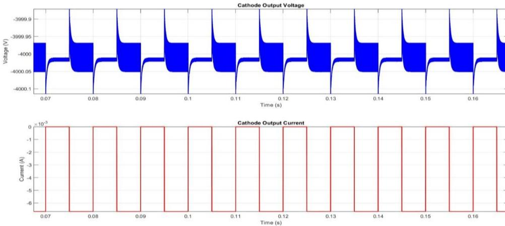
Fig.43: Low PRF Regime of 100Hz with a Duty Ratio of 50% with ACMC and CSA.
