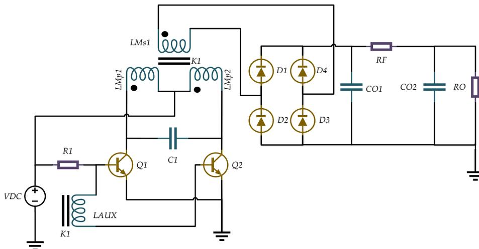
Fig.4: Self-Driven Resonant Oscillator for Ultra-Low Noise, High Voltage Outputs.
