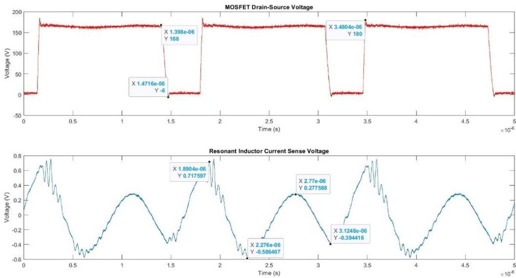
Fig.59: Series Resonant Inductor Current Sense within Multi-Resonant ACF Converter.
