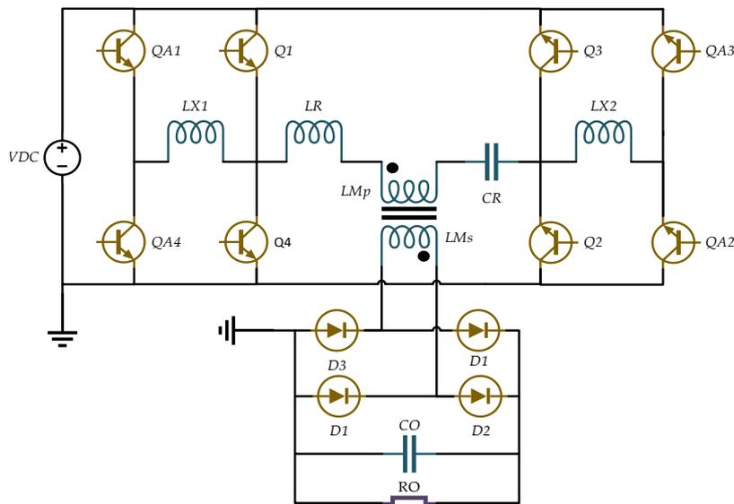
Fig.6: Full Bridge SRC with Phased-Shifted Auxiliary Circuits for No-Load Regulation.
