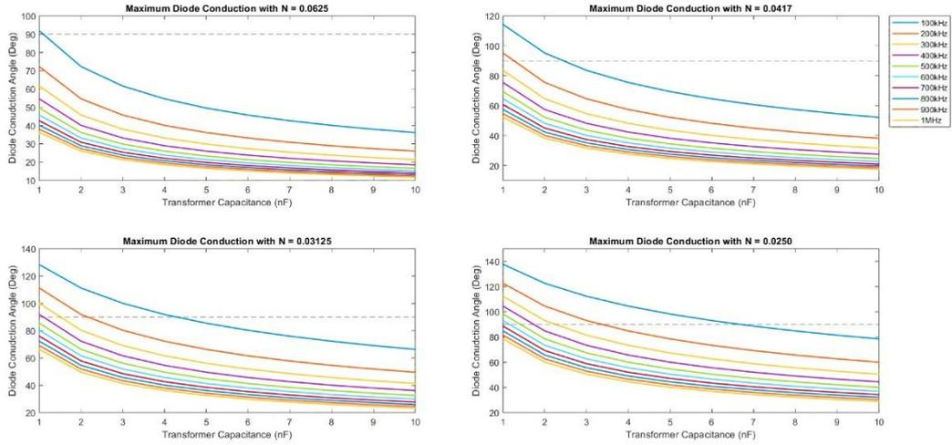
Fig.20: Required Diode Conduction Angles with Different Transformer Turns Ratios and Switching Frequencies for Differing Transformer Parasitic Capacitances with Load Resistance of 600K $\Omega$ .
