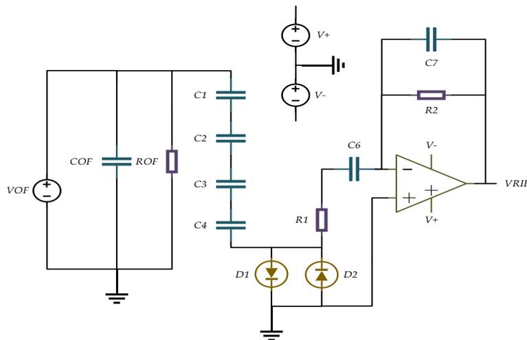
Fig64: Proposed Circuit Implementation for Measurement of AC Voltage Variation on the Critical Cathode Electrode Output.
