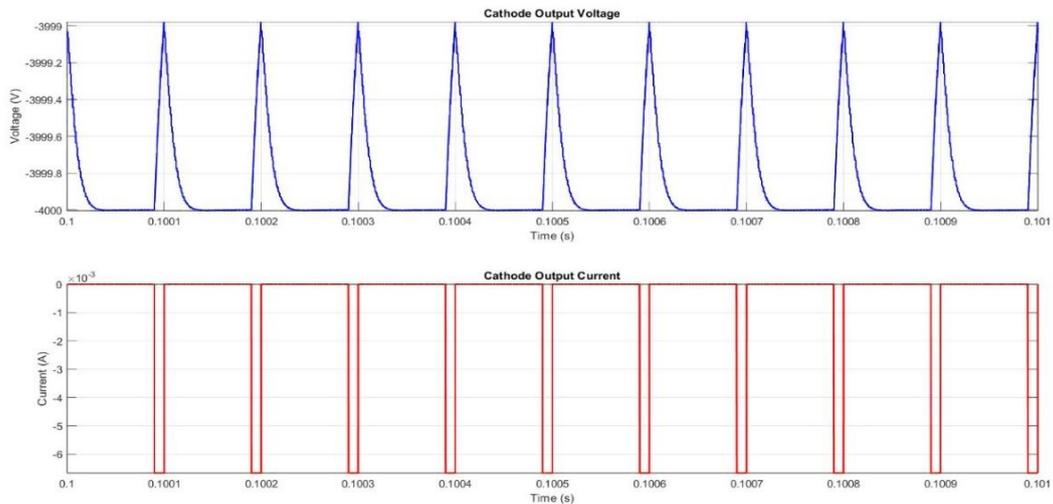
Fig.40: Moderate PRF Regime of 10kHz with a Duty Ratio of 10% with Voltage Mode Control.
