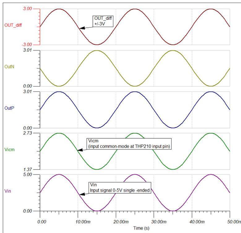
Fig.69: Translation of 0-5VDC Cathode Feedback Voltage to a Differential Output Voltage.
