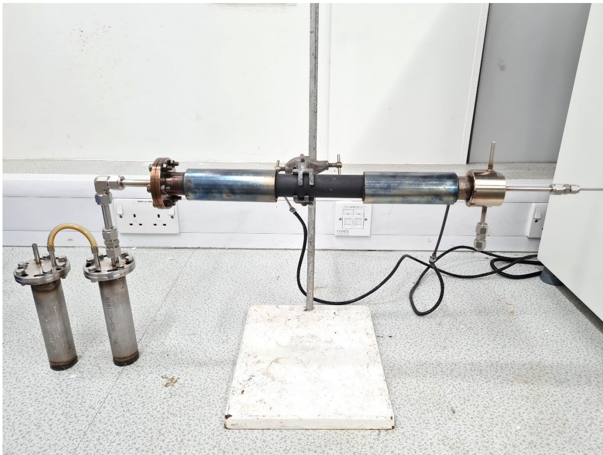
Figure B.1. Pyrolysis system showing reactor, heating elements, and condensers (insulation not shown).
