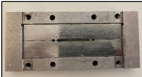
Figure 4-8: Custom split steel mould.
