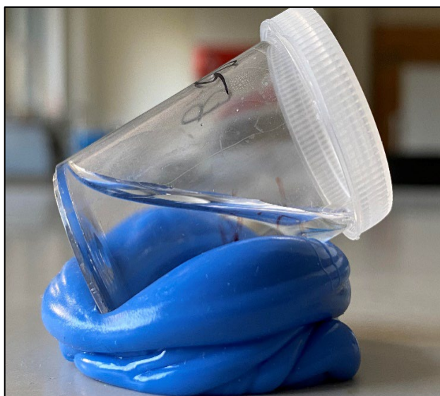
Figure 4-6: Fluoride ion test specimen in 5ml DW
