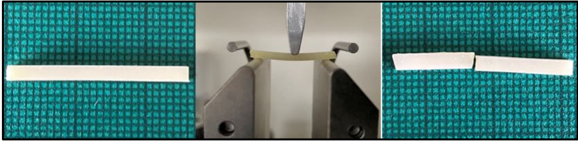
Figure 4-10: 55F sample before (A), During (B) and after (C) FS test.
