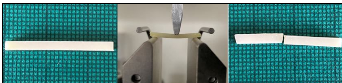
Figure 2: one of the samples before, During and after applying the flexural test.
