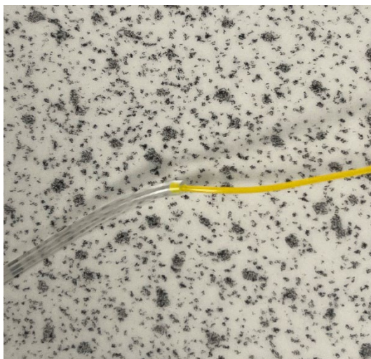
Figure 3-9. Home-made plug to close the external catheter port. (a) a monofilament fishing line (60lb) was inserted inside a polyvinylchloride (PVC) round tube (bore: 0.50mm and wall: 0.50mm).
