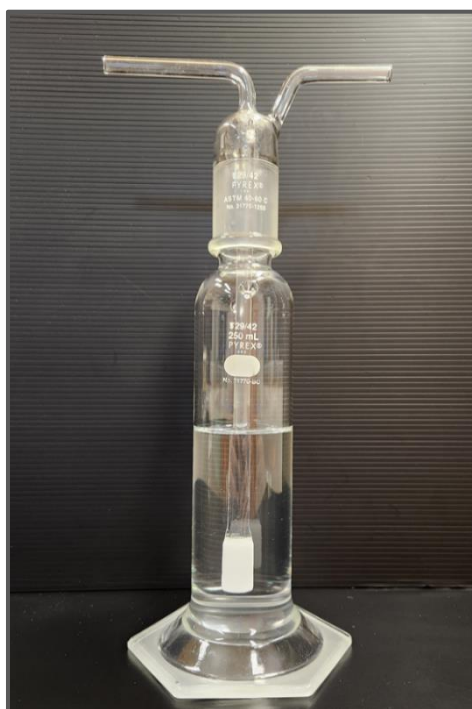
Figure 3-1: The gas bubbling reactor used in this study.
