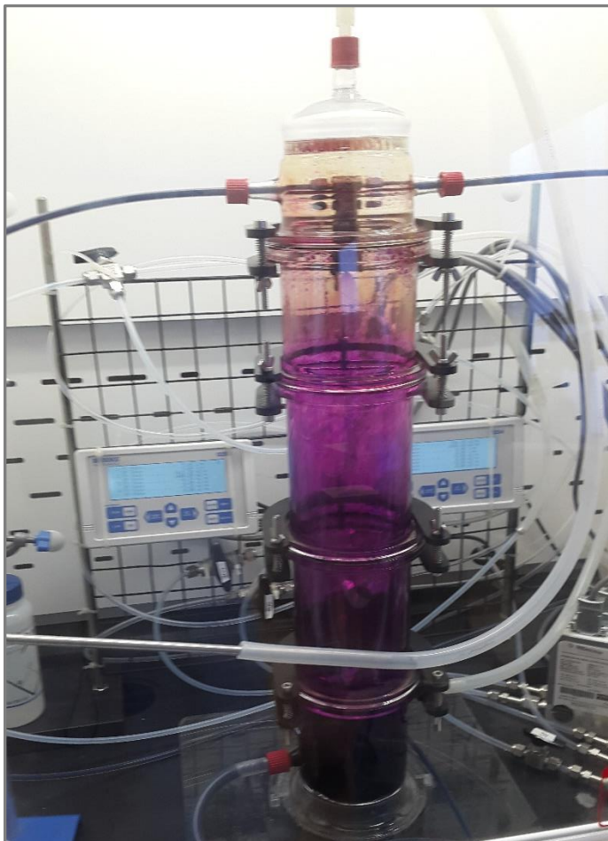
Figure 4-21: The counter-current wet scrubber with \text{KMnO}_4 as the scrubbing liquid. Etching of \text{MnO}_2 precipitates encountered on glass, tubings, nozzle and mist eliminator.
