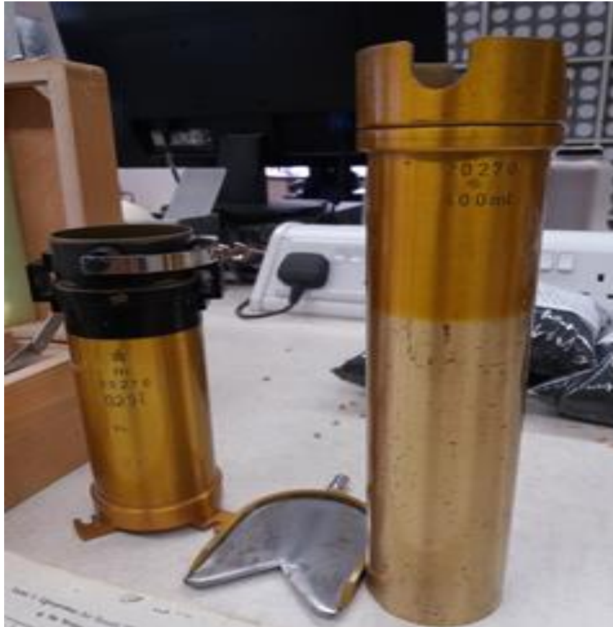
Fig. 4.3 Hectolitre weight measurement using the test weight-chondrometer, including filler, cutter bar and 0.25 L calibrator.
