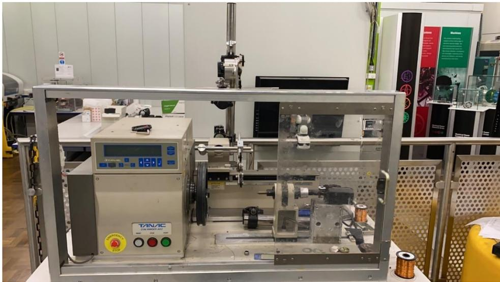
**Figure 7-2: Winding machine**
