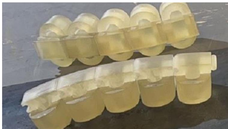
**Figure 7-5: 3D printed tooth units and winding blocks**
