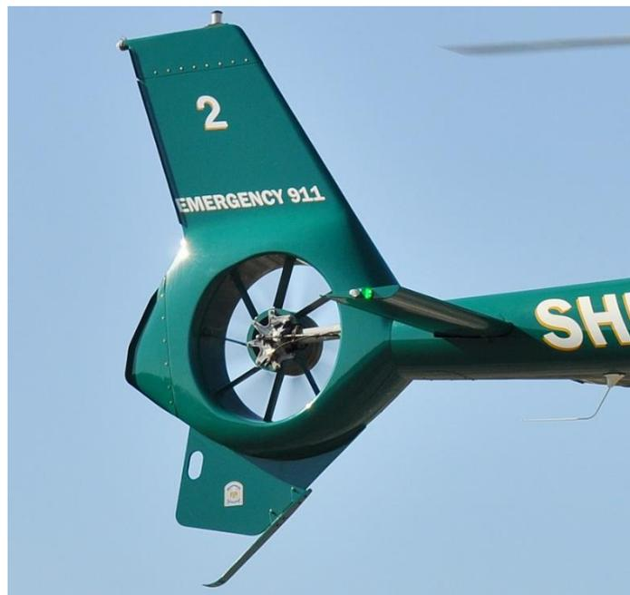
**Figure 2-9: Fenestron tail rotor – EC120B [37]**
