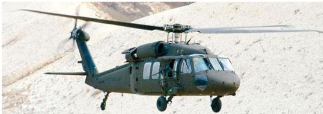
**Figure 2-6: UH-60A single main rotor and tail rotor helicopter**
