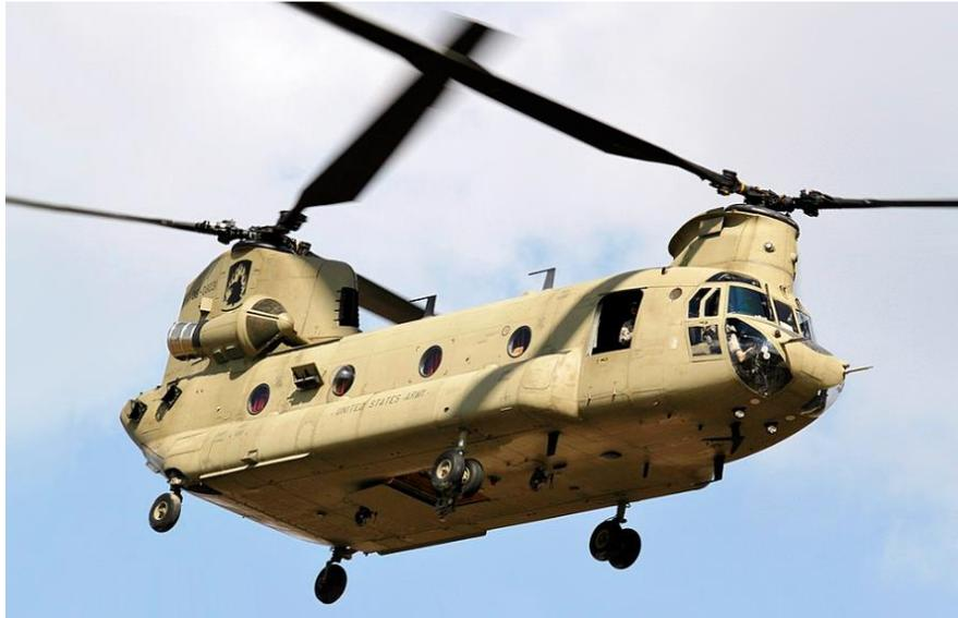
**Figure 2-7: A tandem main rotor helicopter – Boeing CH-47 Chinook**
