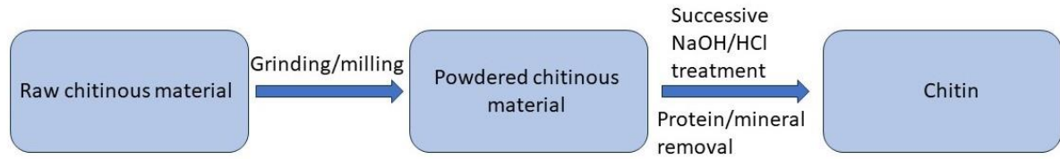
Figure 7 – Basic chemical processing of raw chitin rich material to produce chitin.
