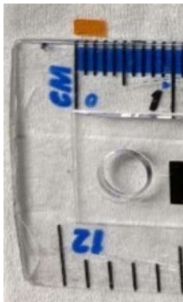
Figure 4.14 Image of MAPbBr 3 single crystal formed by IR-cell of liquid method with dimension of 4×2 mm.
