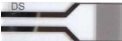
Figure 6.1. Interdigitated Pt on glass microelectrodes (DRP-G-IDEPT10). The sample is deposited on the right grey part of the electrode.
