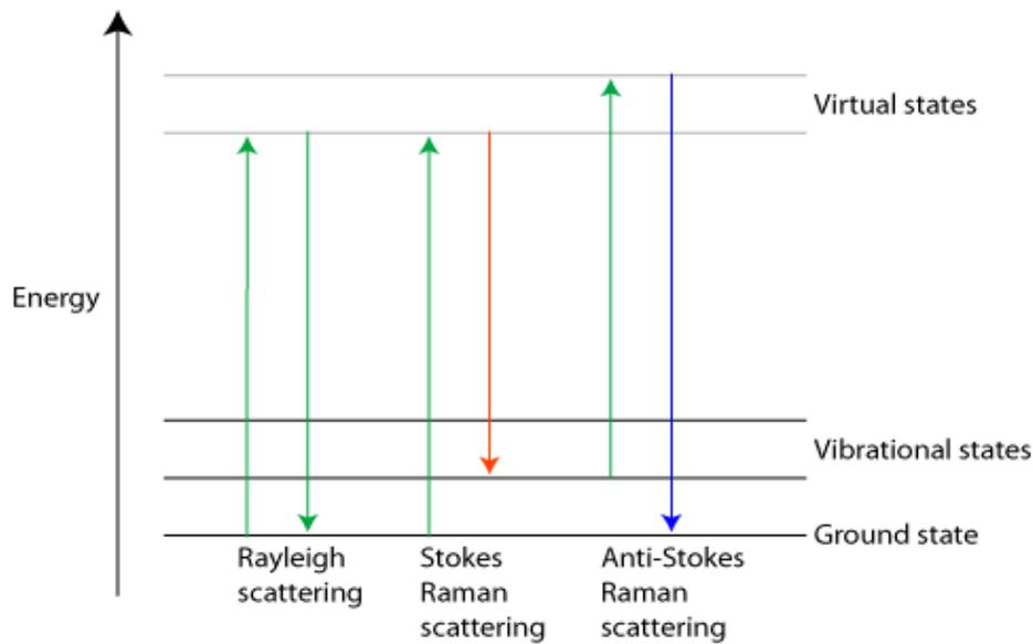
Figure 4.11: Demonstrates the three Raman scattering processes of Rayleigh, Stokes, and Anti-Stokes under the light-material interaction. The upward and downward shift in energy is due to obtaining or losing energy from a phonon to a phonon or unsteady state in the material.
