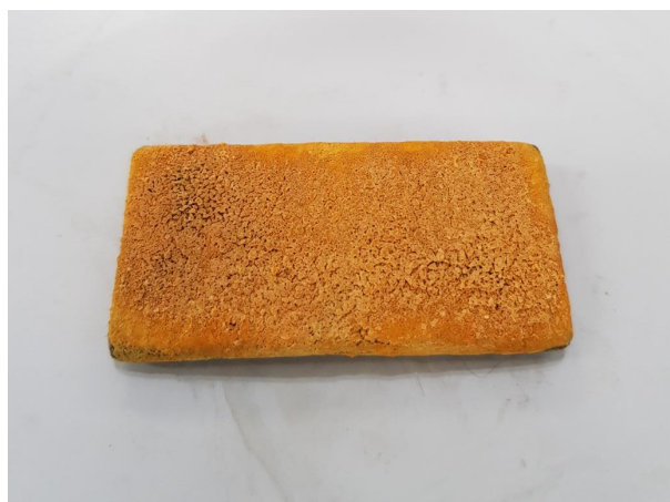
Figure 5.19 Photo of a 2.5 cm x 5 cm piece of carbon felt coated in ca. 0.3 g ferrocene. This was achieved by dissolving the ferrocene in ethanol, soaking the carbon felt in this solution and evaporating the solvent.
