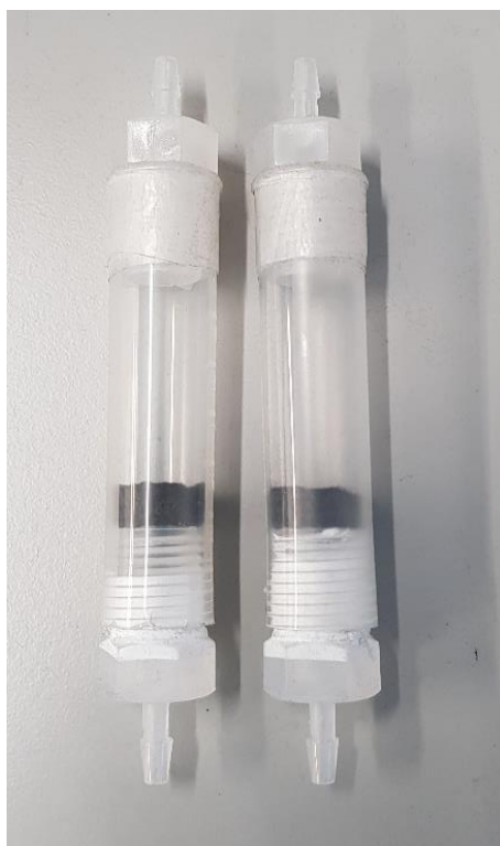
Figure 5.14 Booster cartridges with connectors for tubing and fitted pieces of carbon felt to retain the booster material during experiments.
