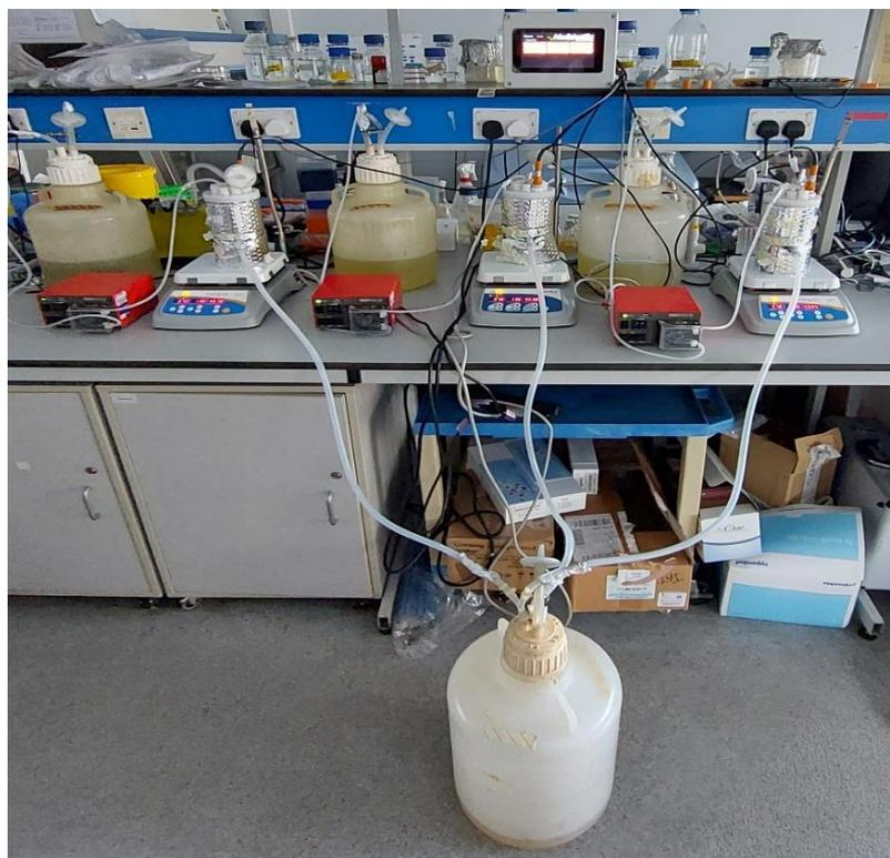
**Figure 2.3** Setup of the CDC reactors. Each CDC reactor, positioned on top of a magnetic stirrer hot plate, was connected to its own carboy containing 6 L of AFMC medium and fed using a peristaltic pump. All reactors were run over the course of 9 days.
