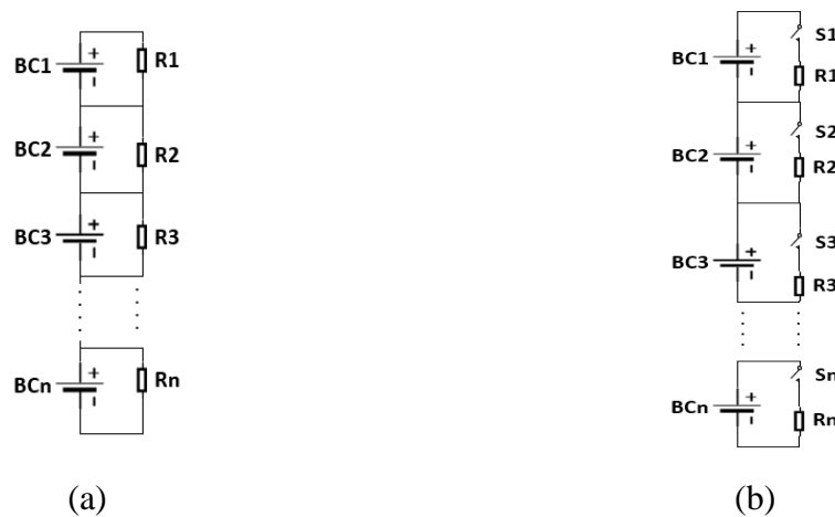
Figure 2.8: Dissipative Balancing Methods, (a) Fixed Shunt Resistor (b) Switched Shunt Resistor
