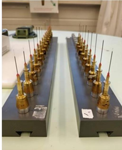
Figure 2.5 **Photographs from ESRF.** a) Reactor system set up at ESRF. b) Capillaries loaded with powdered samples used for room temperature scans.
