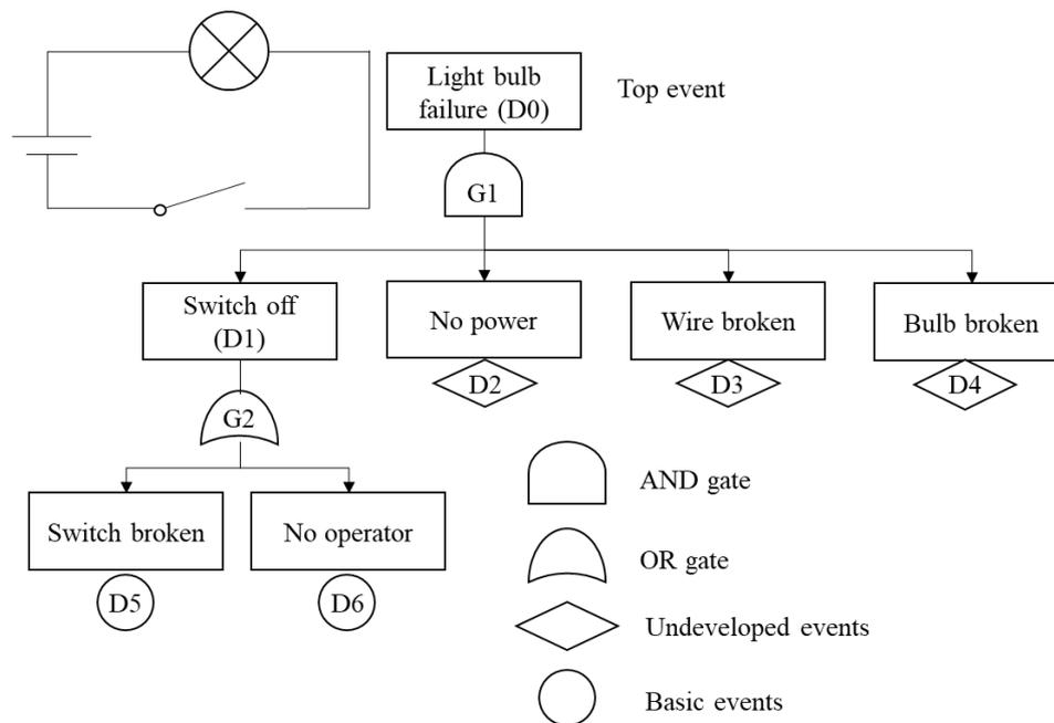
Figure 15. Fault tree analysis for light bulb does not light up.
