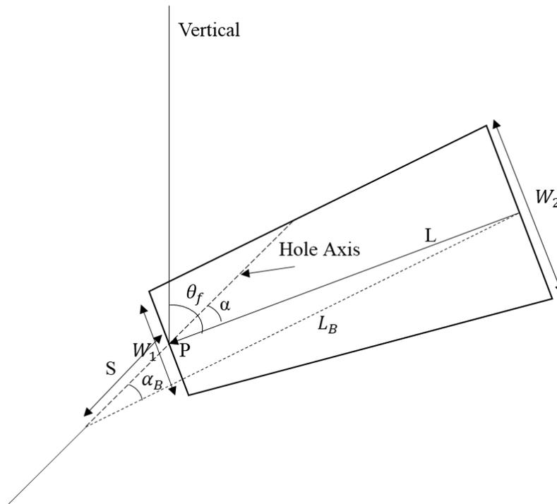
Figure 36. Sketch a jet fire's flame geometry (Chamberlain, 1987).
