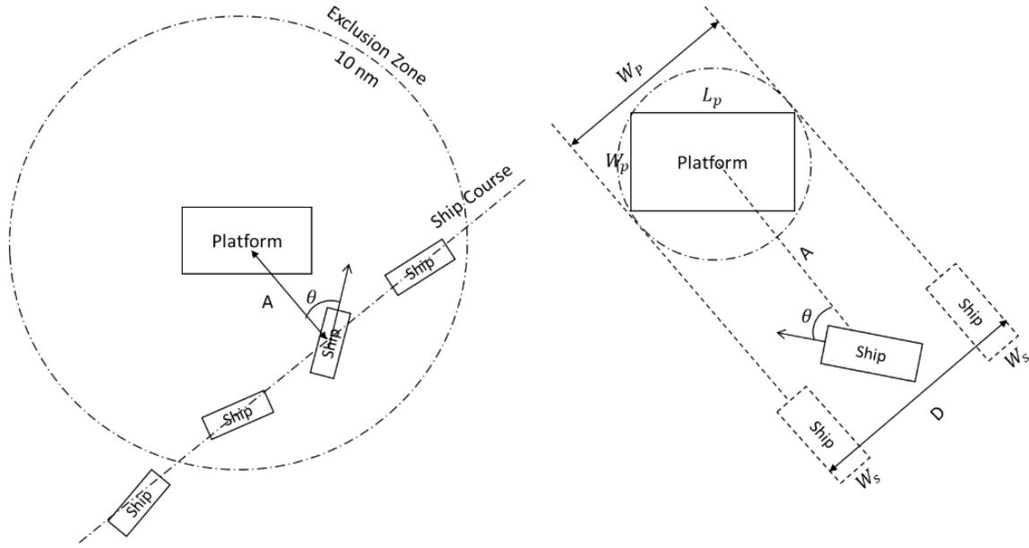
Figure 34. Collision geometry diagram.
