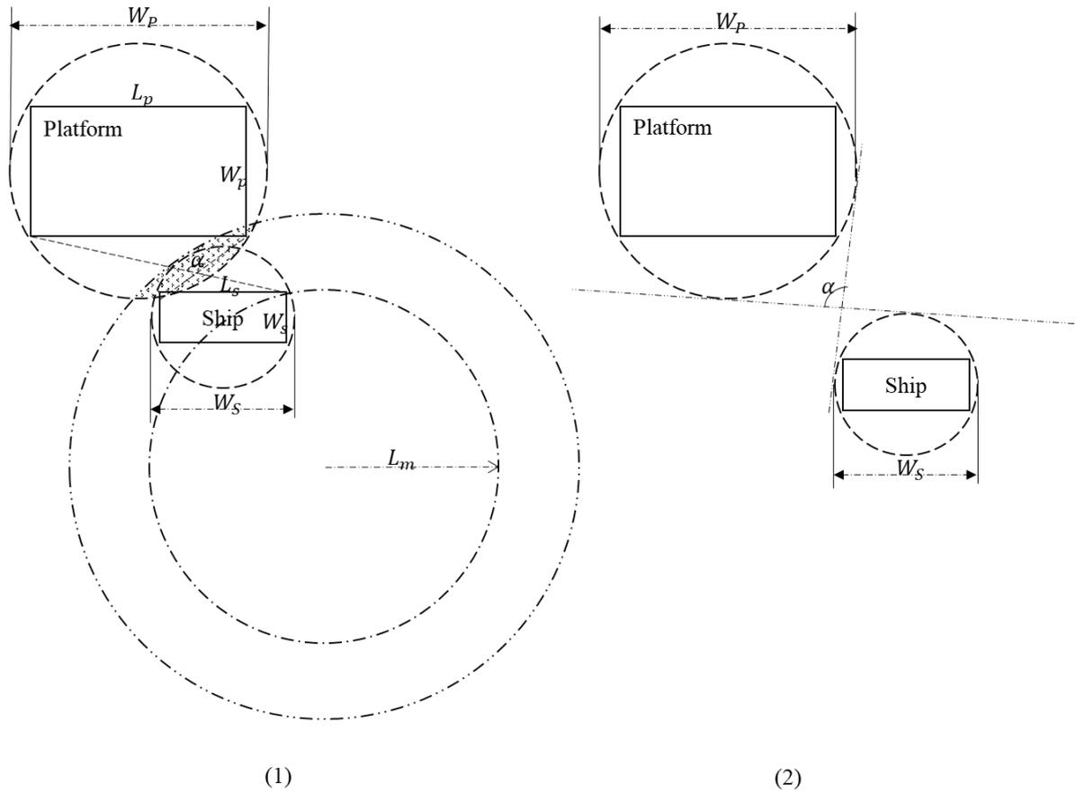
Figure 35. Ship and Platform Collision Geometry Schematic.
