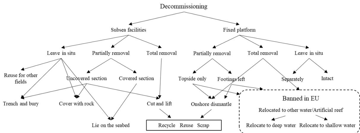
Figure 2. Decommissioning options for fixed platforms and subsea facilities (Fowler et al., 2014; Ekins et al., 2006)
