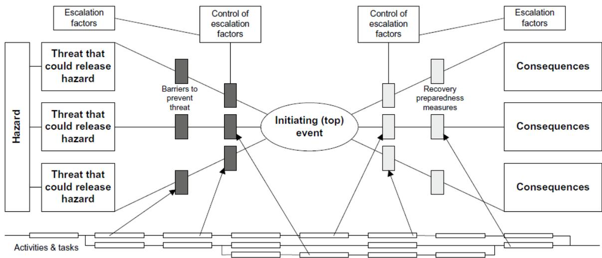
Figure 14. A typical bow-tie diagram.
