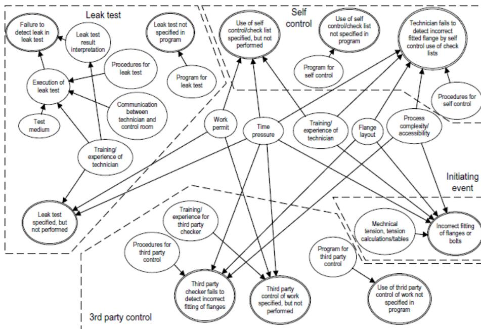
Figure 19. BBN case example for pipe leakage (Røed et al., 2009).
