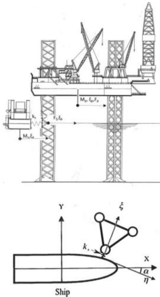
Figure 37. Vessel collision with platform.
