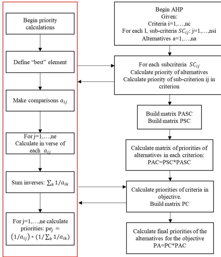
Figure 6. Steps to use AHP, PASC is Priorities of the Alternatives in each Sub-criterion, PSC is the Priorities of the Sub-criteria for each Criterion, PAC is the Priorities of the Alternatives in each Criterion, PC is the Priorities of each Criterion, PA is the final Priorities of the Alternatives (Leal, 2020).
