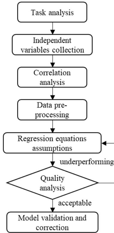
Figure 22. Top-down framework model regression analysis procedure.
