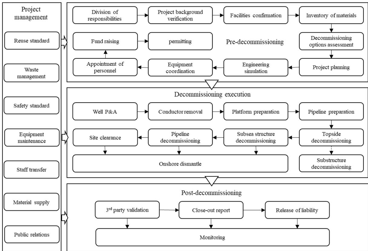
Figure 3. General decommissioning procedures for offshore oil and gas facilities (Fam et al., 2018; Ruivo & Morooka, 2007)
