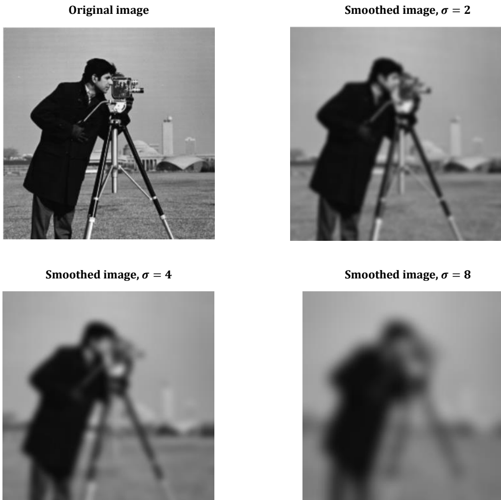
Figure 7.11: Application of Gaussian smoothing filters to an image by specifying a scalar value for sigma.
