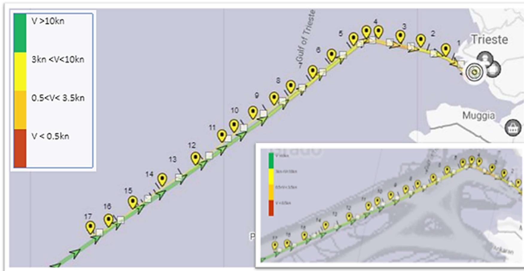
Figure 6.3: Speed and manoeuvring distance analyses (Chapter 4, figures 4.4 and 4.5.) on the example of one containership trajectory. The smaller image presents the same track position on the ship density map.
