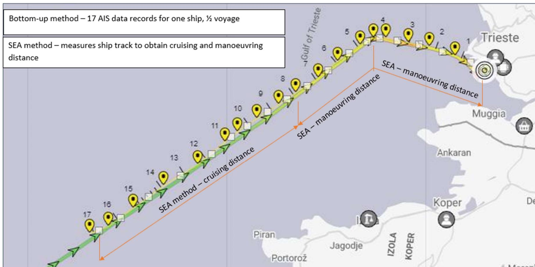
Figure 5. 8: Schematic presentation of voyage data acquisition using the Bottom-up model vs SEA method (Marine Traffic, 2020)
