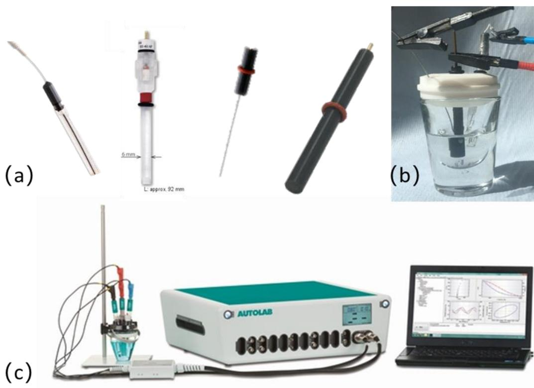
Figure 3.3 Experiment set-up for electrochemical analysis. (a) The electrodes (from left to right: Ag/AgCl reference electrode, ACE, counter electrode, GCE), (DropSens 2020) (b) the glass cell and (c) the Autolab potentiostat-galvanostat used in research (DropSens 2020).
