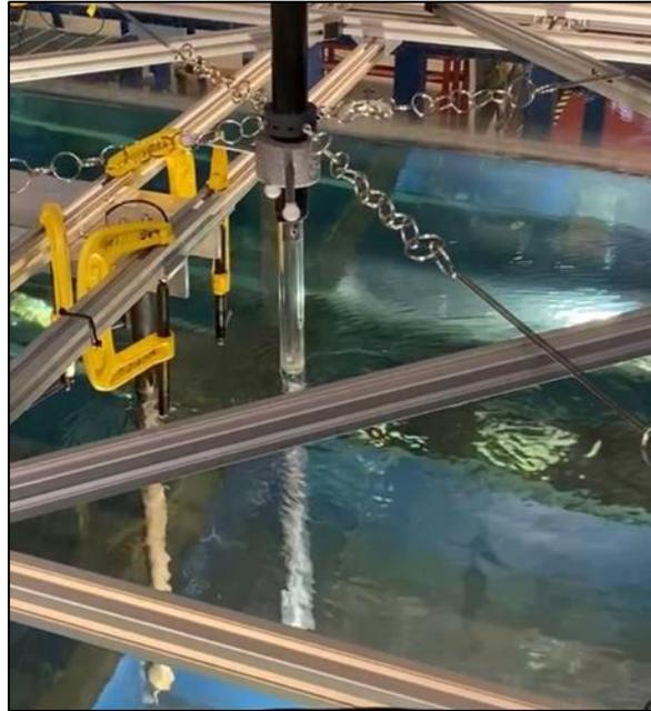
Figure 5-13: Photograph of staggered WIV tests for a flexibly mounted cylinder behind a stationary upstream cylinder.
