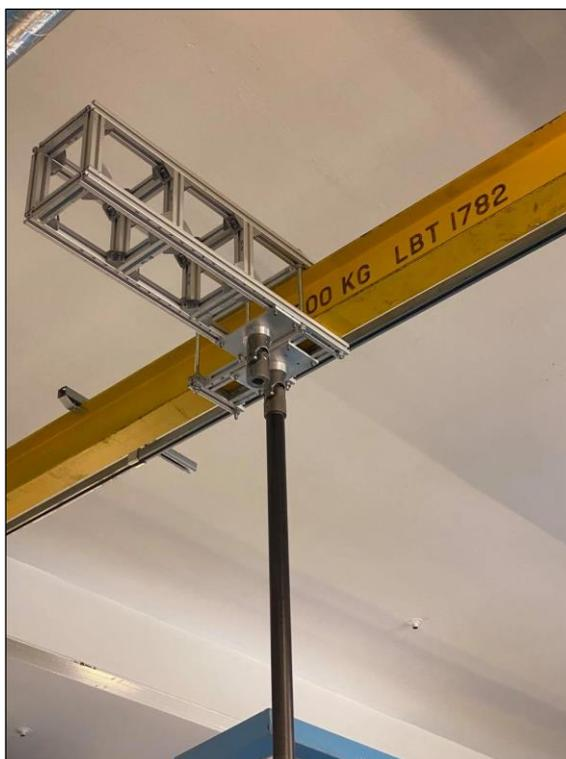
Figure 4-2: Attachment of pendulum systems to a beam over the Hydrodynamics Laboratory. View of the universal joints and mounting carriage system. Sliding carriage structure's greater length is aligned with the flow and WWCT tank. Photo taken at the single cylinder flow measurement phase with the downstream cylinder's carbon fibre tube in place.
