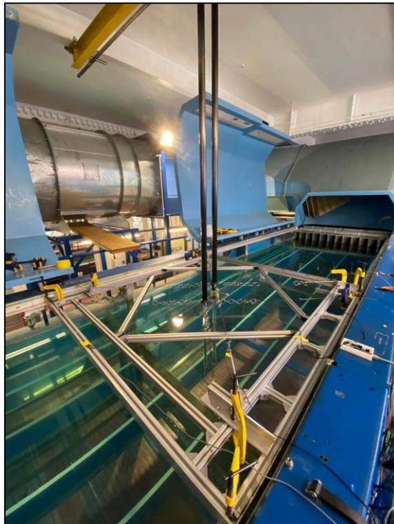
Figure 6-1: Photograph of the free-free pair of tandem identical cylinders, frame and pendulum systems.
