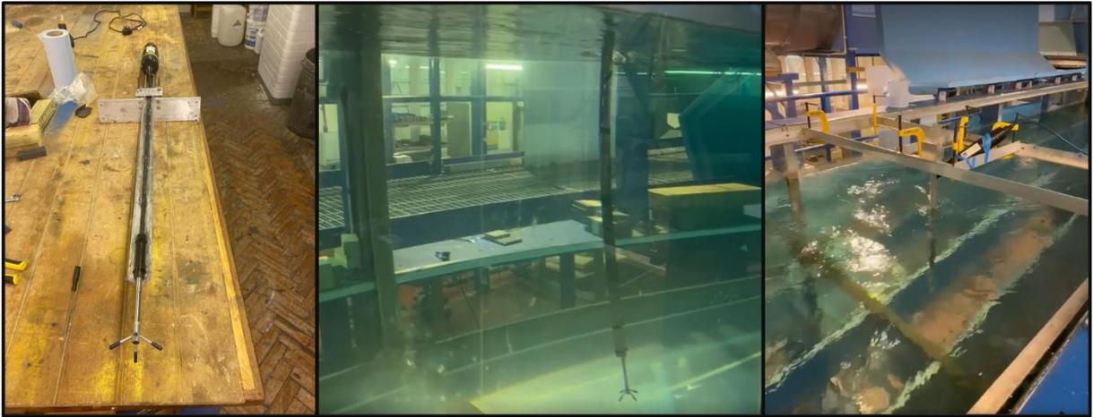
Figure 4-5: Nortek's Vectrino 3D acoustic velocimeter and mounting system. WWCT central tank current flow measurements at different depths.
