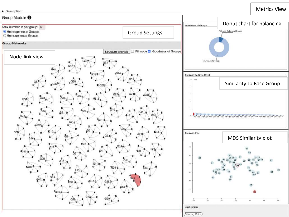
Figure 7-1 Overview of group view. The main view of Group module includes 3 parts, Group setting, Node-link view, and Metric view. Group setting allows to change Group type and appearance of given views. Node-link view represents groups formed. Metric view includes 3 different metrics to visually show the goodness of formed groups in terms of homogeneity and heterogeneity. (User Knowledge Modelling data was used.)
