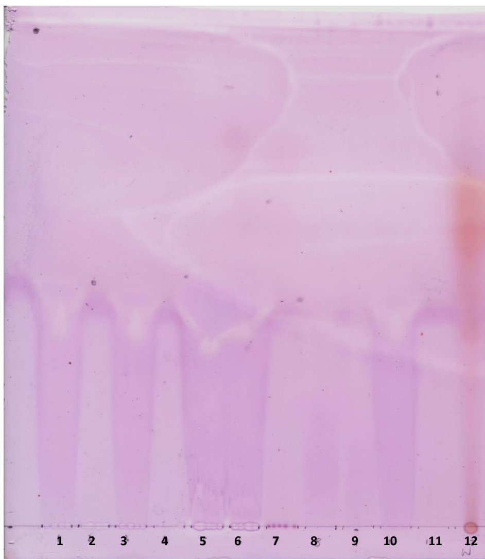
Figure 2.5. TLC with 10 fractions of NCPPB. 4369, and a sugar standard. The plate had two ascents (2 x 8hrs) in BAW. Each lane had a different fraction or sugar standard loaded onto it, with lane 9 and 11 being left blank. Lanes present in the TLC plate were loaded with the following:
