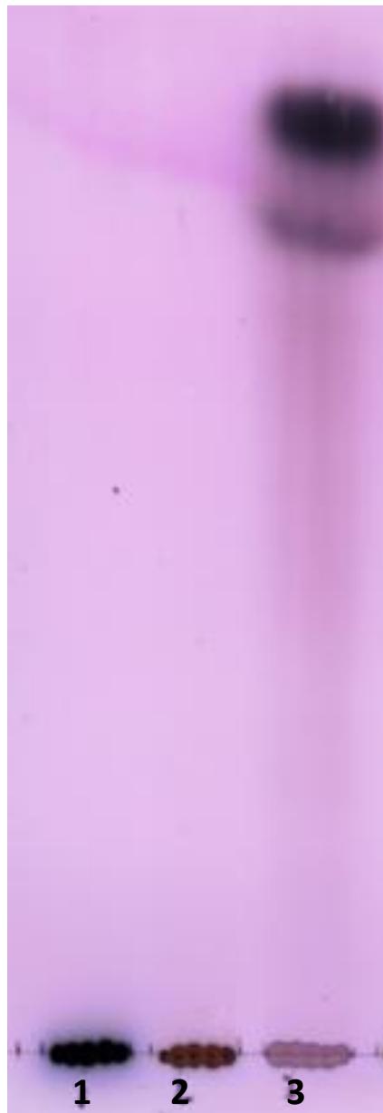
Figure 2.6. TLC with CDTA and NaOH extracts of NCPPB. 4369, and a xylan polysaccharide standard serving as a positive control. Two ascents (2 x 8hr) in BAW. Lanes present in the TLC plate were loaded with the following:
