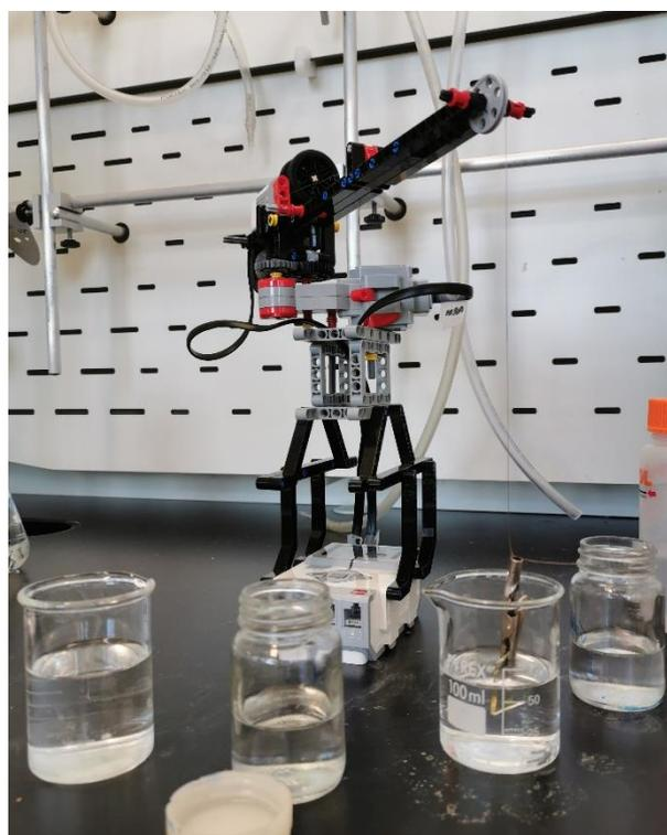
**Figure 12:** Photograph of the one of the first iterations of the LEGO SILAR robot.
