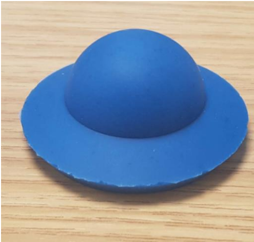
Figure 6.11 The first design of novel pressuriser with a smaller excavating surface of radius 25mm.
