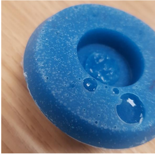
Figure 6.7 A number of bubbles can be seen on the backside of the novel pressuriser. As this is a non-functional surface it is not critical that it is free from imperfections.
