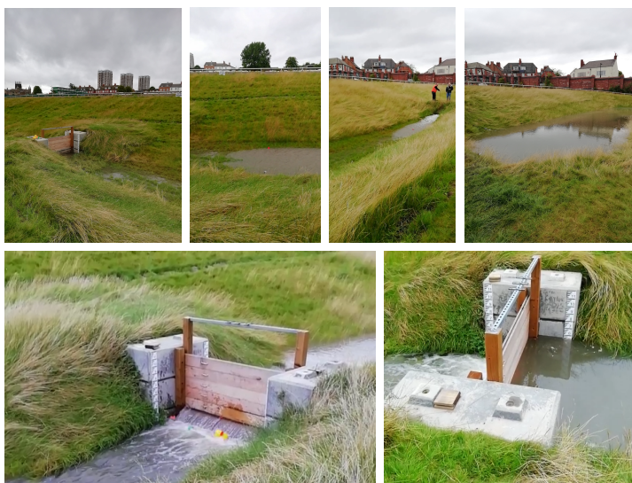
Figure 1.5: Leaky barrier experiment in the swale at Newcastle University's National Green Infrastructure Facility. Flow from right to left.
