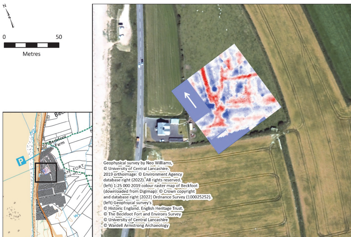
Figure 5.11: Results from 2011 resistivity survey, part of an undergraduate dissertation (Adapted from: Williams, 2011, p. 16).
