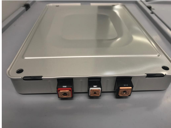
Figure 6.1: Battery module from first generation Nissan Leaf EV (li-ion)
